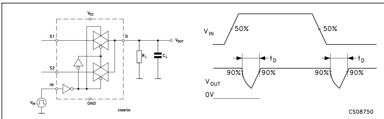
CHARGE INJECTION ( $V_{GEN}=0V$ ,  $R_{GEN}=0\Omega$ ,  $R_L=1M\Omega$ ,  $C_L=100pF$ )
