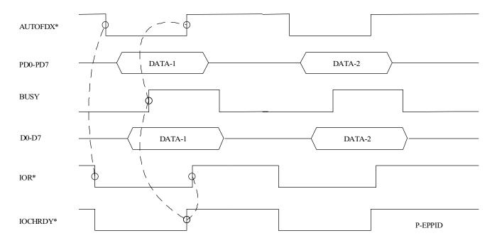
EPP MODE ( MODE 100, ADDRESS READ, INPUT MODE )
