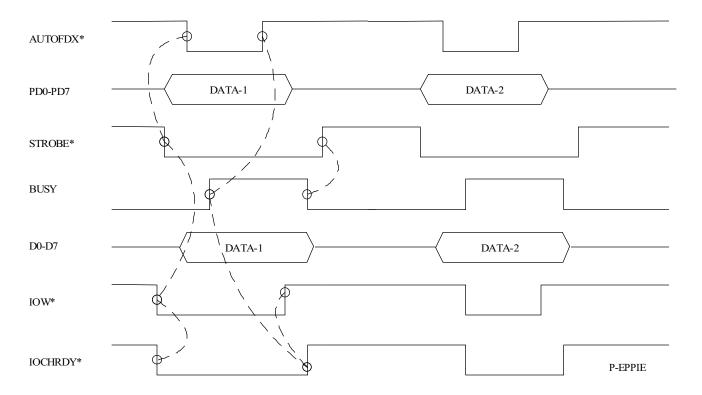
EPP MODE ( MODE 100, WRITE ADDRESS, OUTMODE )
