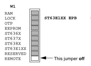
For ST63E1XX EPBs, remove the REMOTE jumper in the W1 jumper bank.
