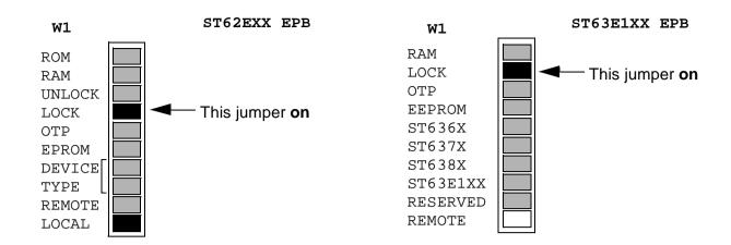
To prevent the device from being ever read-protected, set the UNLOCK jumper. This function is available for devices with the OPTION byte (ST62E2XX only).
