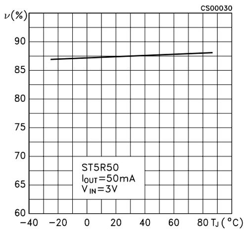
Figure 6: Efficiency vs Temperature
