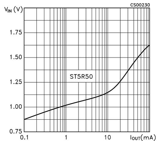
**Figure 20: Minimum Input Voltage vs Output Current**
