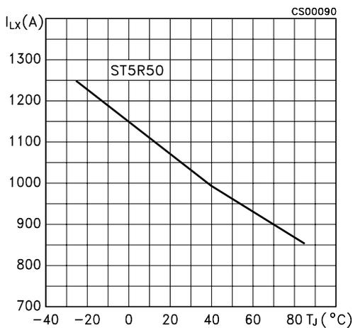
**Figure 14: Lx Switching Current Limit vs Temperature**
