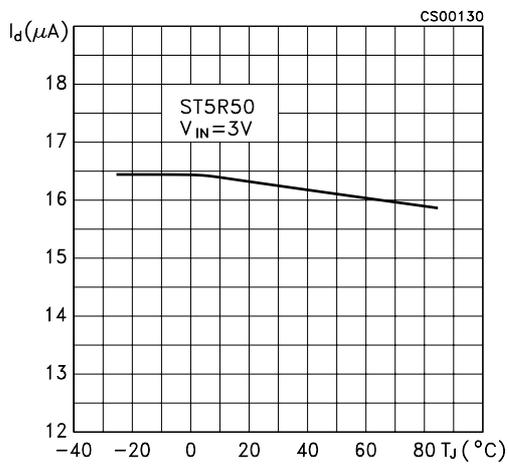
Figure 26: No Load Input Current vs Temperature
