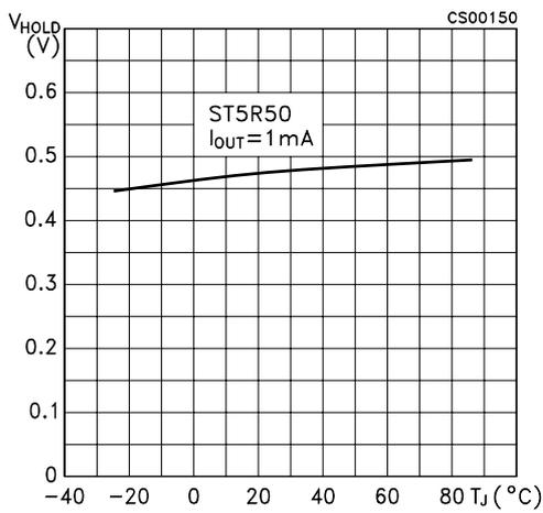
Figure 24: Hold-on Voltage vs Temperature
