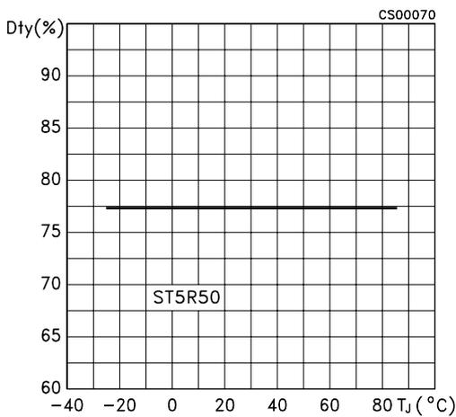
**Figure 12: Oscillator Duty Cycle (@ MAX Freq.) vs Temperature**
