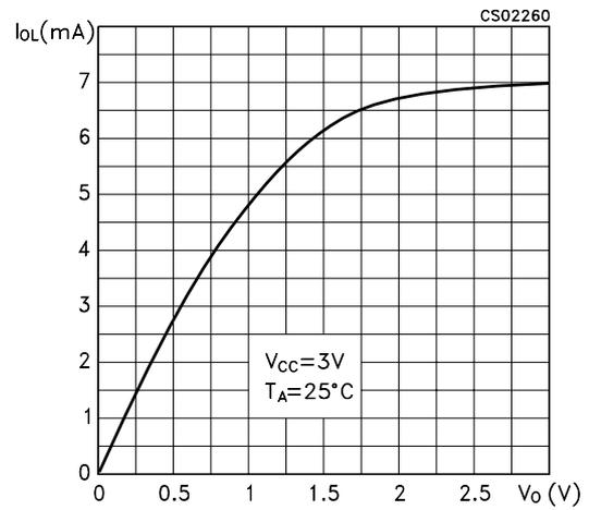
**Figure 2 :** Driver Voltage Transfer Characteristics for Receiver Inputs
