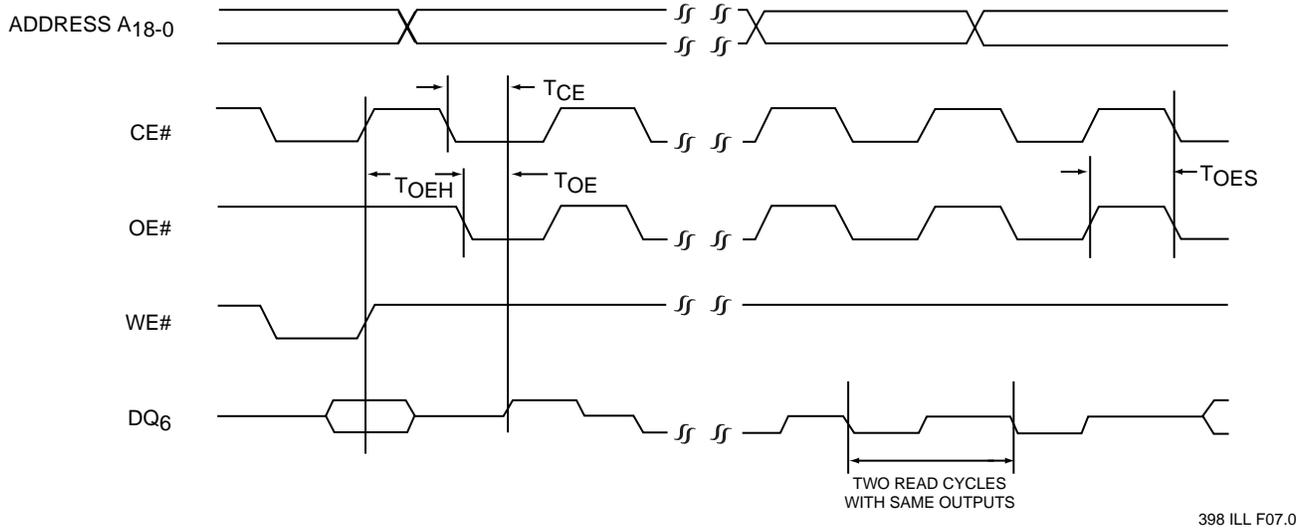
FIGURE 8: TOGGLE BIT TIMING DIAGRAM
