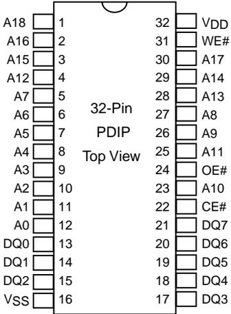
**FIGURE 2: PIN ASSIGNMENTS FOR 32-PIN PDIP**
