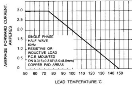
FIG. 2 - MAXIMUM AVERAGE FORWARD CURRENT RATING
