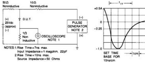
FIG. 1 - REVERSE RECOVERY TIME CHARACTERISTIC AND TEST DIAGRAM
