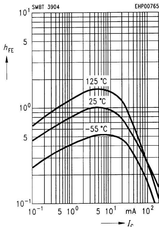
**Short-circuit forward current transfer ratio**  $h_{21e} = f(I_c)$
