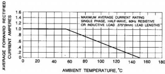
Fig. 3 - MAXIMUM AVERAGE FORWARD CURRENT RATING
