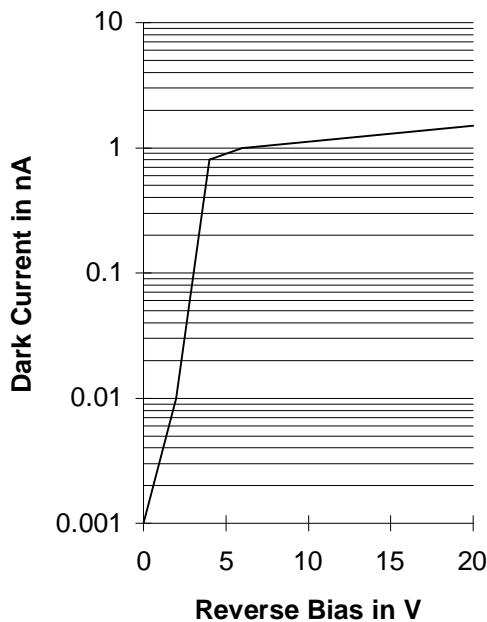
**Dark Current of PIN Diode  $I_R = f(T_A)$**
