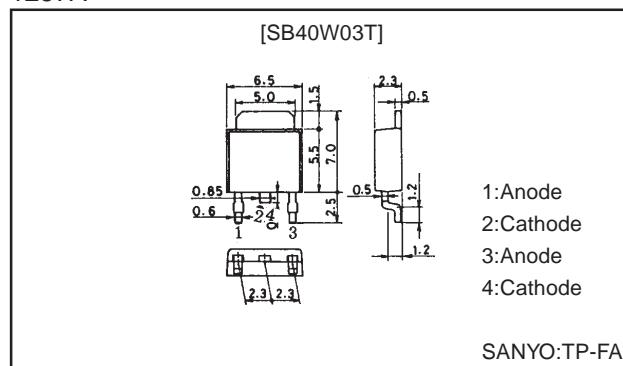
**Specifications****Absolute Maximum Ratings at  $T_a = 25^\circ\text{C}$  (Value per element)**
