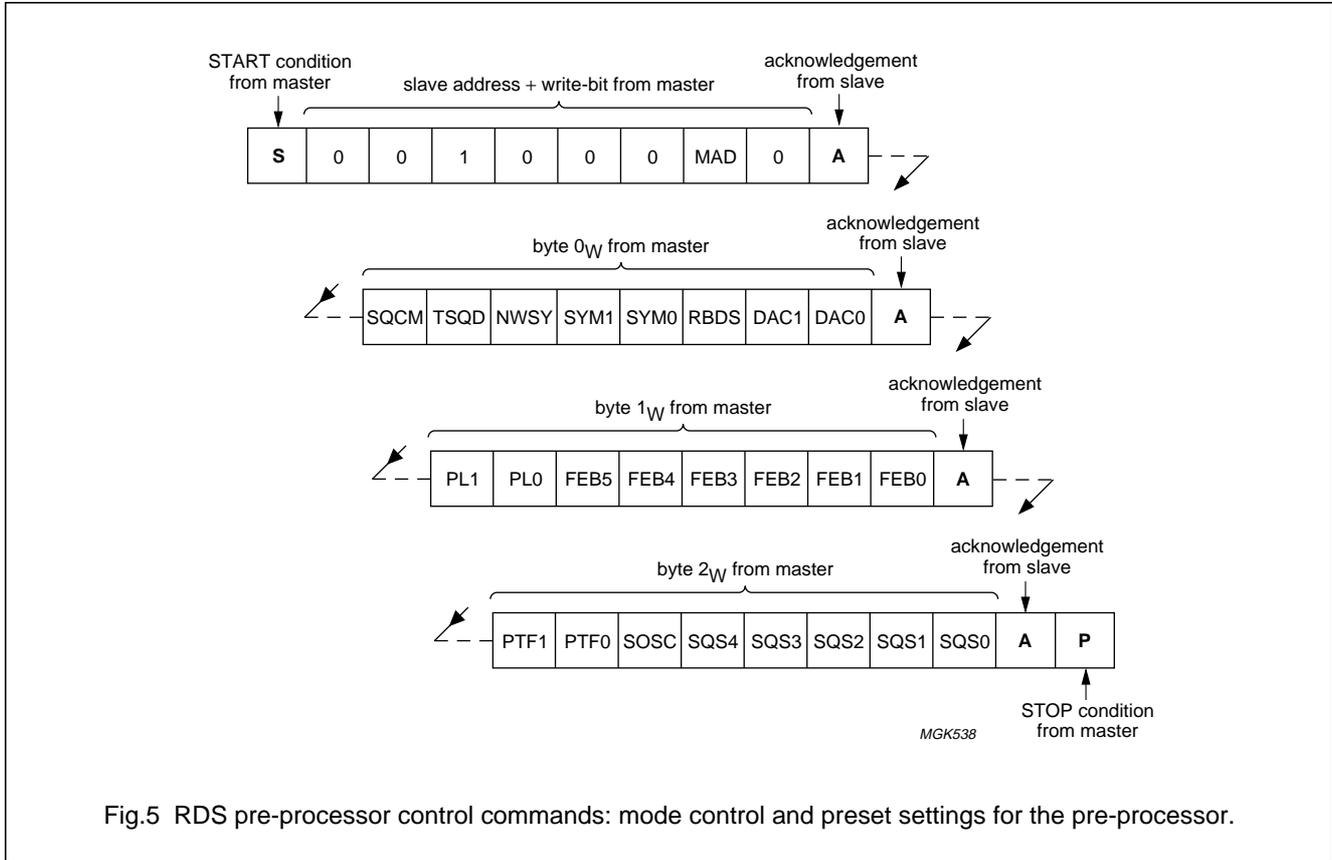
Fig.5 RDS pre-processor control commands: mode control and preset settings for the pre-processor.
