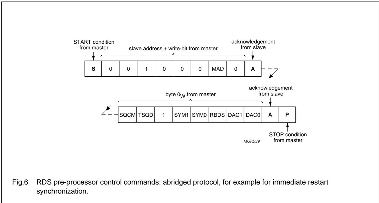
Fig.6 RDS pre-processor control commands: abridged protocol, for example for immediate restart synchronization.
