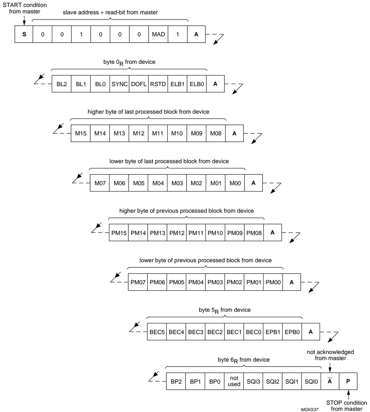
Fig.7 Data output protocol (RDS data output).
