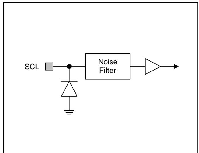
Figure 6-4. Pin Circuit Type 2
