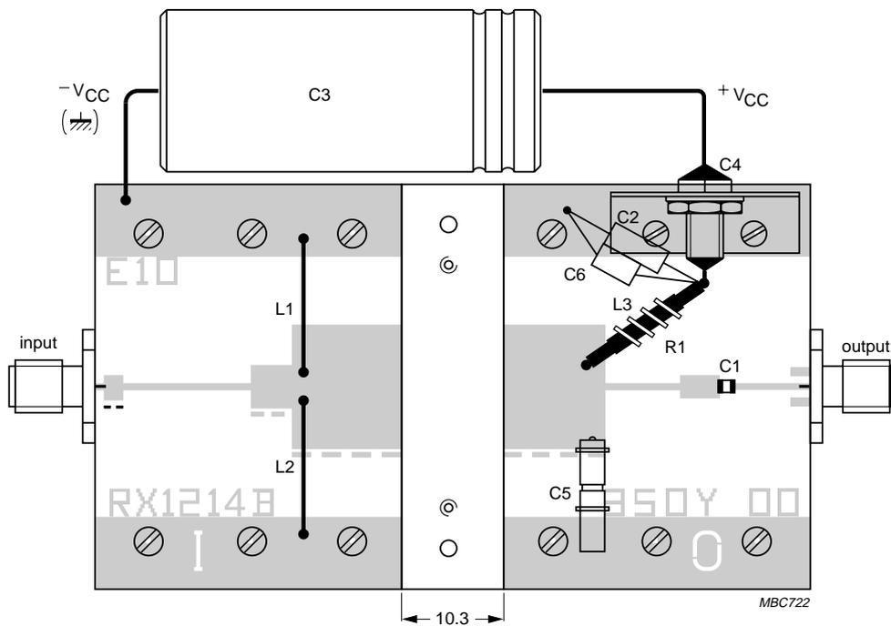
Fig.3 Broadband test circuit.
