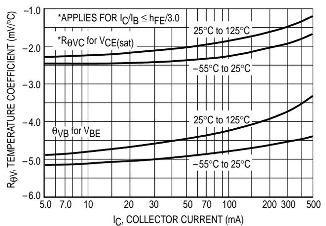
Figure 6. Temperature Coefficients
