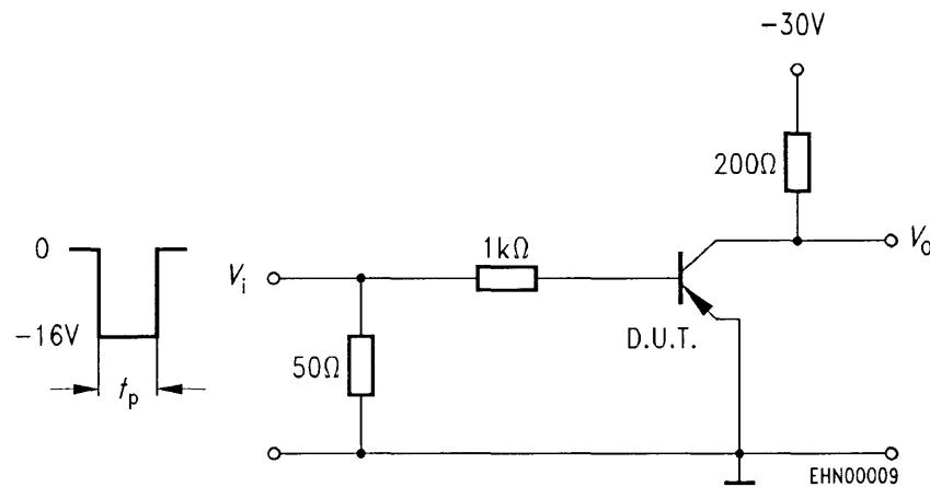
**Input waveform and test circuit for determining storage, fall and turn-off time**Turn-off time when switched to  $-I_{Con} = 150 \text{ mA}$ ; $-I_{Bon} = 15 \text{ mA}$  to cut-off with  $+I_{Boff} = 15 \text{ mA}$
