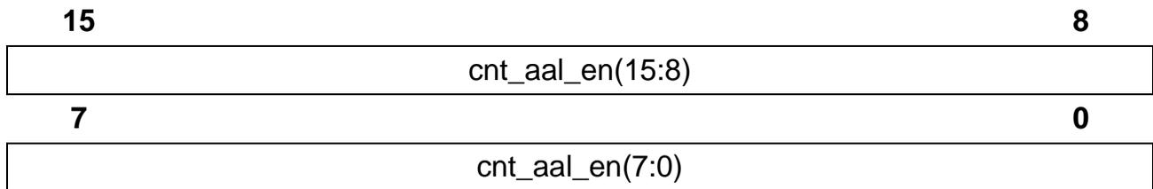
cnt\_aal\_en(15:0) OAM-counter enable for AAL ports
