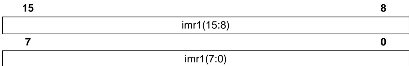
A bit set in this register, masks the corresponding interrupt in isr1.
