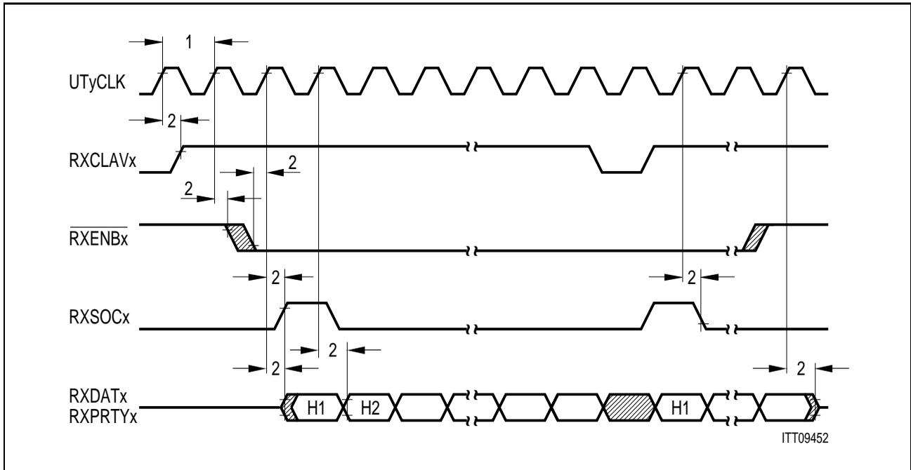
Figure 29 Utopia receive interface timing diagram
