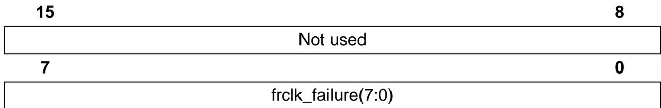
frclk\_failure(7:0)      FRCLK clock failure on port(7:0)
