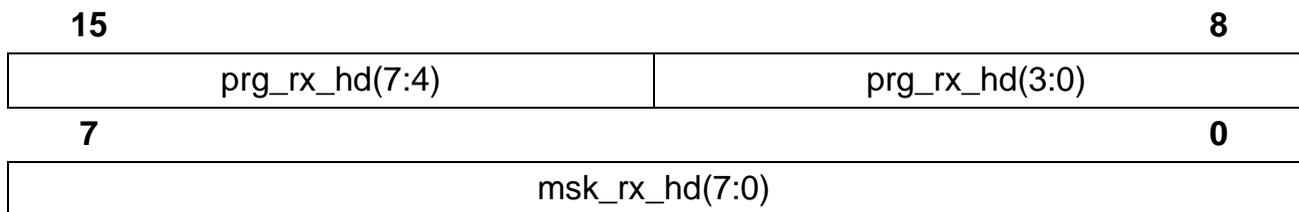
prg\_rx\_hd(7:4)           Programmable rx idle/unassigned cell header octet 1 bits (7:4)
