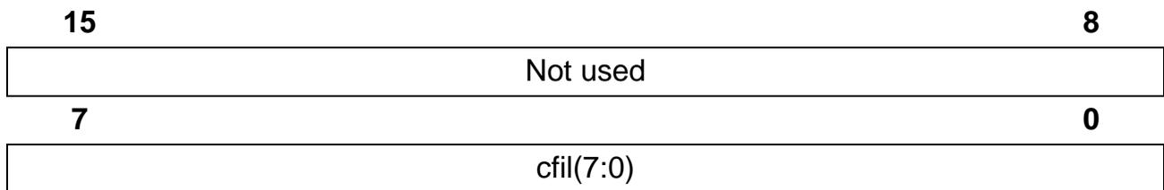
cfil(7:0)            Dummy fill octet in partially filled cells
