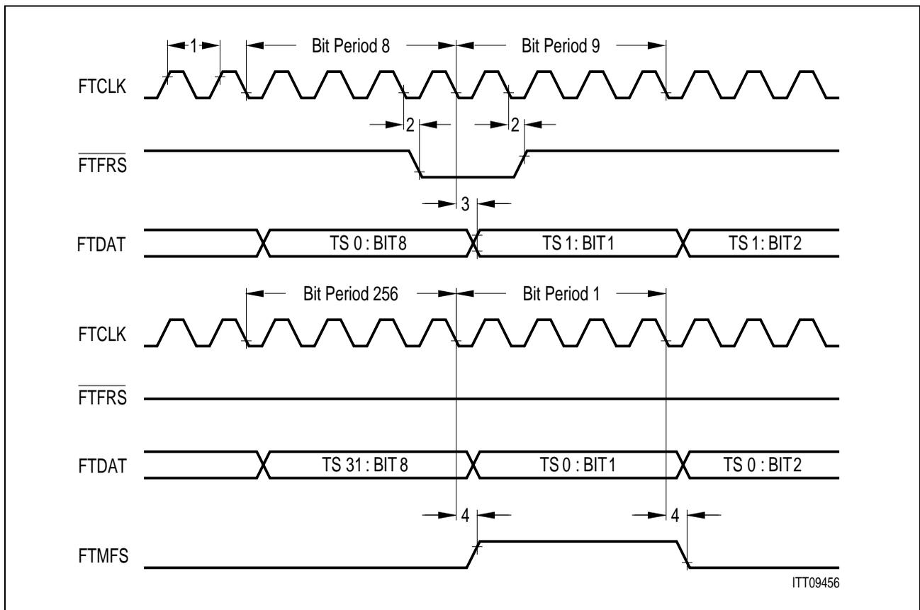
Figure 33 Framer transmit interface timing diagram
