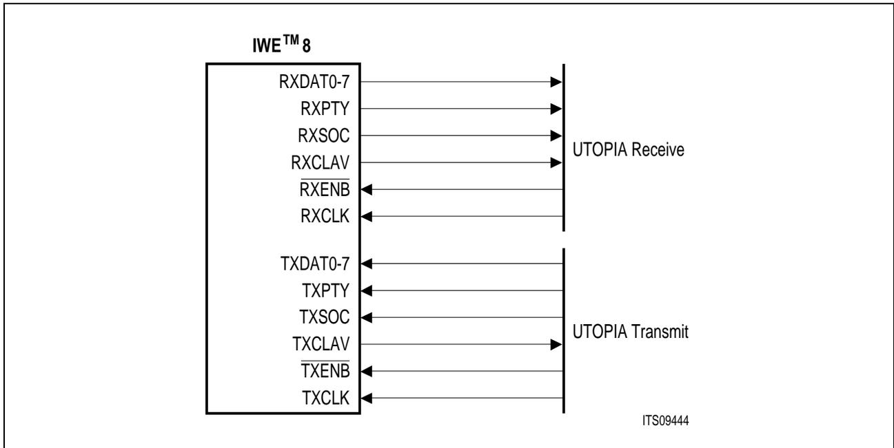
Figure 12 UTOPIA receive and transmit interfaces.
