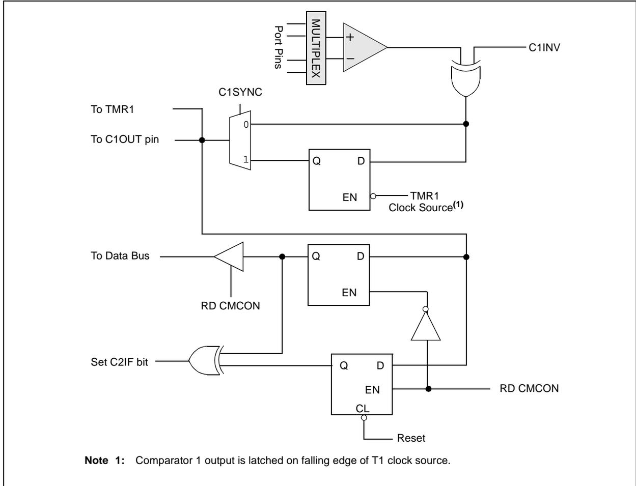
**FIGURE 7-6: PIC16F636 COMPARATOR C1 OUTPUT BLOCK DIAGRAM**
