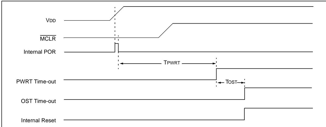
**FIGURE 11-5: TIME-OUT SEQUENCE ON POWER-UP (DELAYED  $\overline{\text{MCLR}}$ )**
