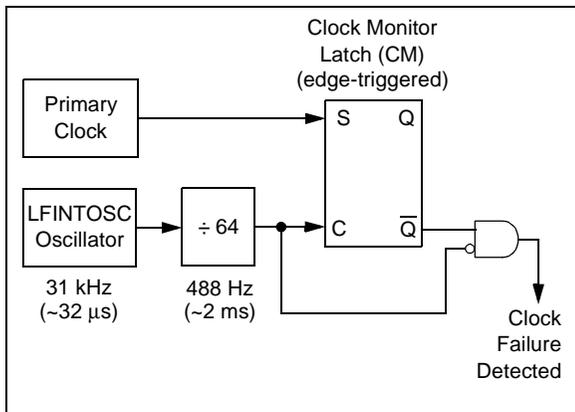
The FSCM function is enabled by setting the FCMEN bit in the Configuration Word register (Register 11-1). It is applicable to all external clock options (LP, XT, HS, EC, RC or I/O modes).
