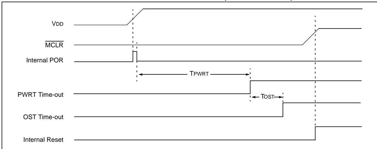
**FIGURE 11-6: TIME-OUT SEQUENCE ON POWER-UP ( $\overline{\text{MCLR}}$  WITH VDD)**
