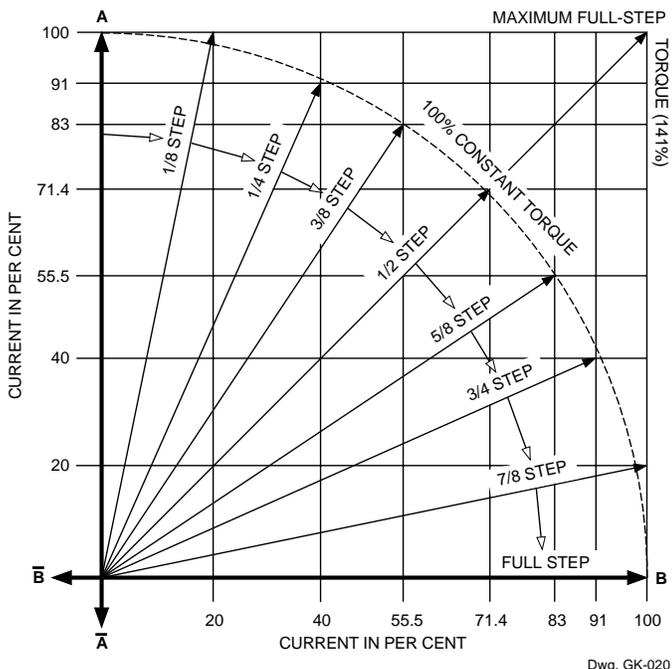
Figure 2 — Current/Displacement Vectors
