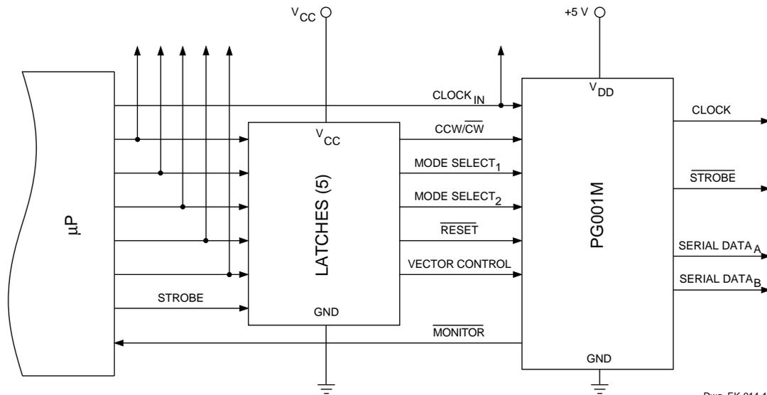
Figure 6 — A Latched Input-Bus Configuration
