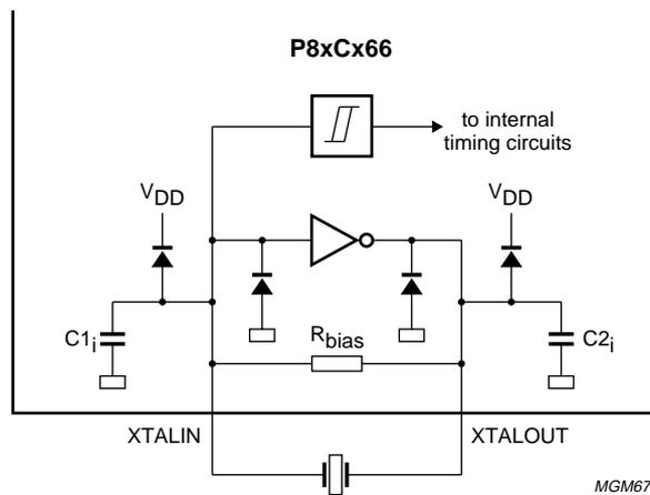
Fig.14 Standard oscillator.
