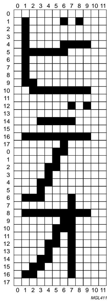
Fig.42 Combination of two font cells in a vertical direction.
