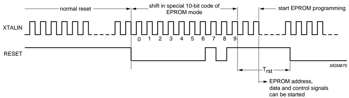
Fig.47 Sequence to enter EPROM programming mode.
