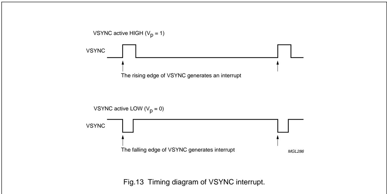
Fig.13 Timing diagram of VSYNC interrupt.
