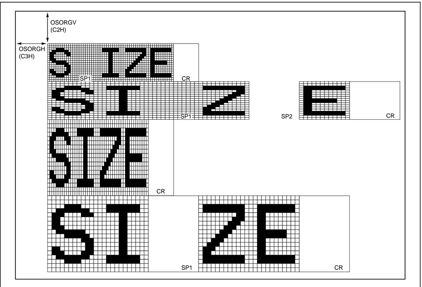
Fig.28 An example of flexible display format (Split space off).
