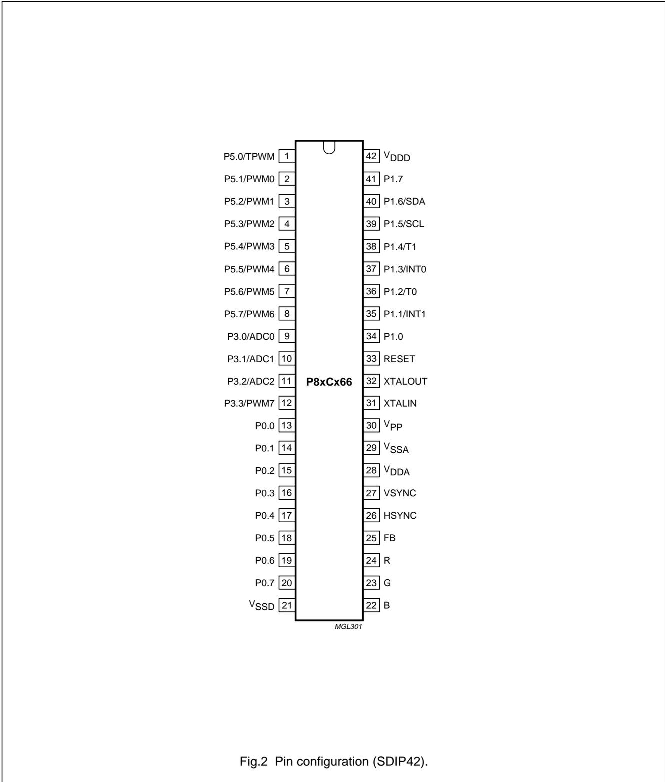
Fig.2 Pin configuration (SDIP42).
