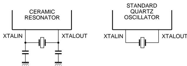
Fig.15 Alternative oscillator configurations.
