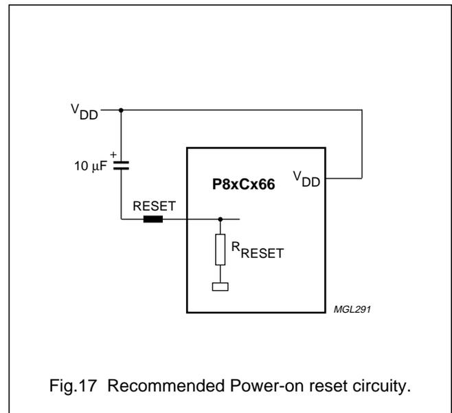
Fig.17 Recommended Power-on reset circuitry.
