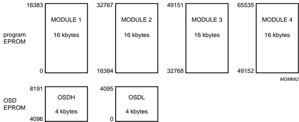
Fig.46 On-chip EPROM structure for the P87C766.
