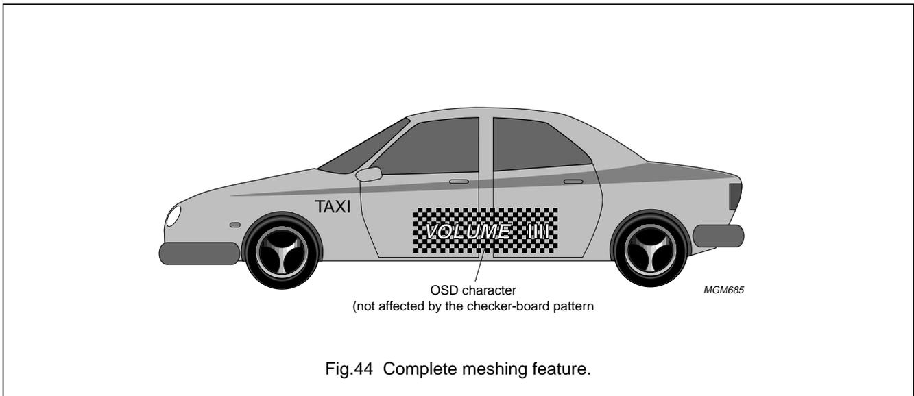
Fig.44 Complete meshing feature.
