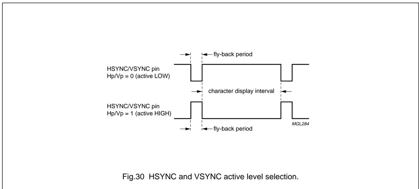
Fig.30 HSYNC and VSYNC active level selection.
