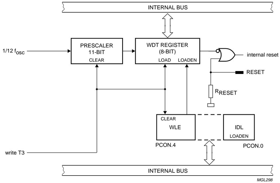
Fig.8 Block diagram of the Watchdog timer.
