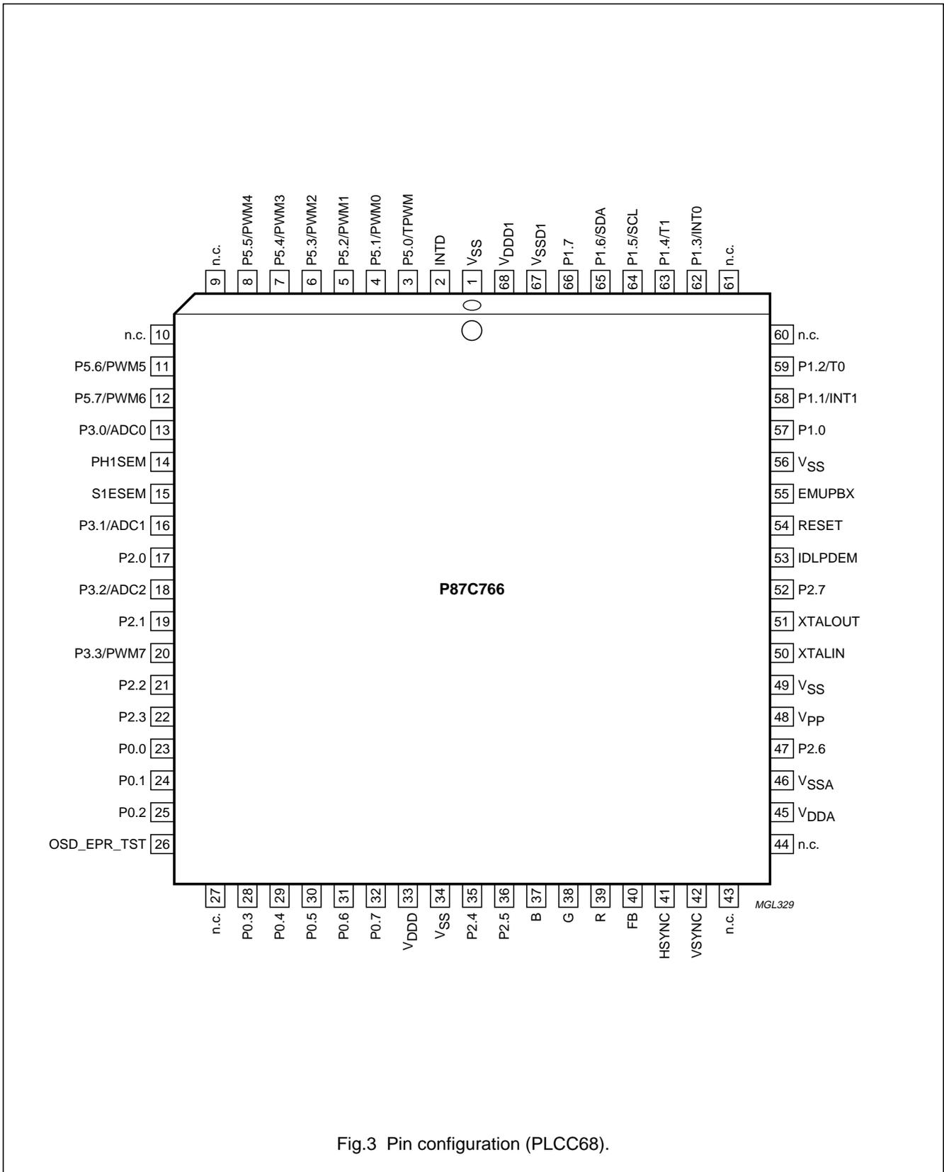
Fig.3 Pin configuration (PLCC68).
