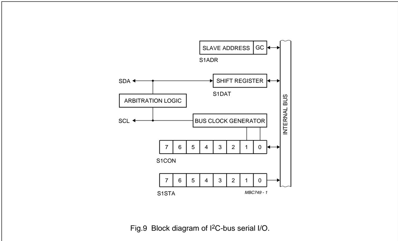
Fig.9 Block diagram of I<sup>2</sup>C-bus serial I/O.
