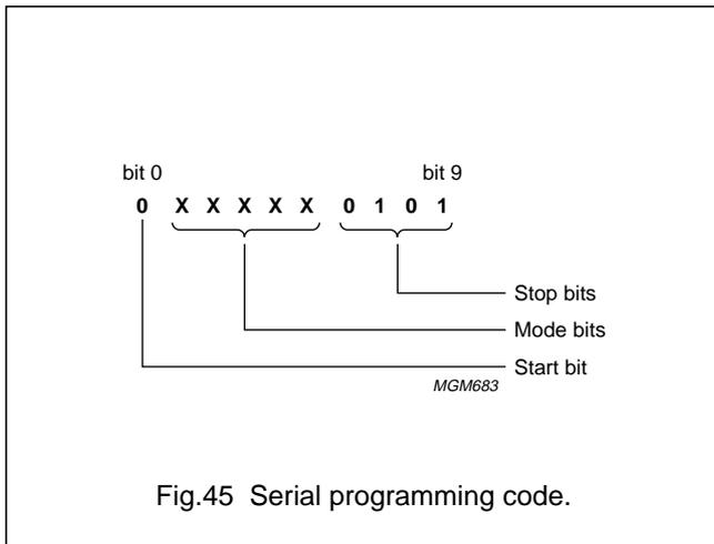
Fig.45 Serial programming code.
