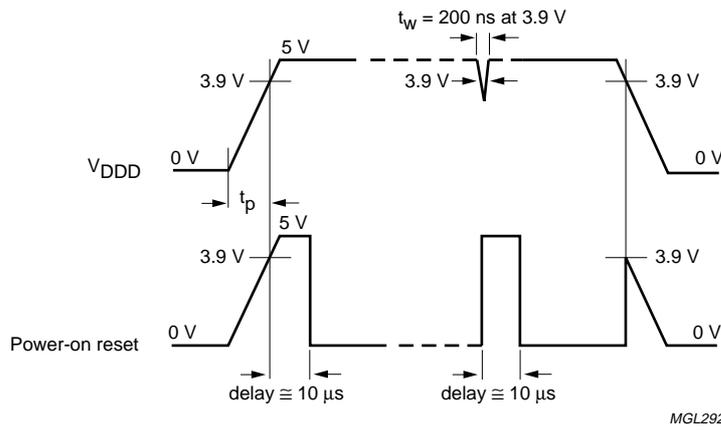
Fig.18 Power-on reset switching level.
