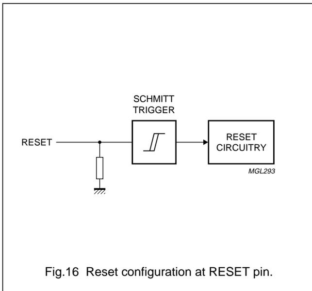
Fig.16 Reset configuration at RESET pin.
