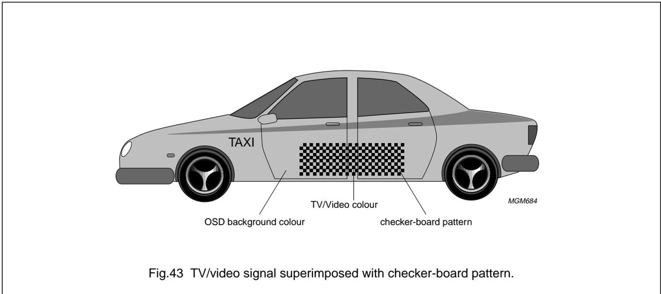
Fig.43 TV/video signal superimposed with checker-board pattern.
