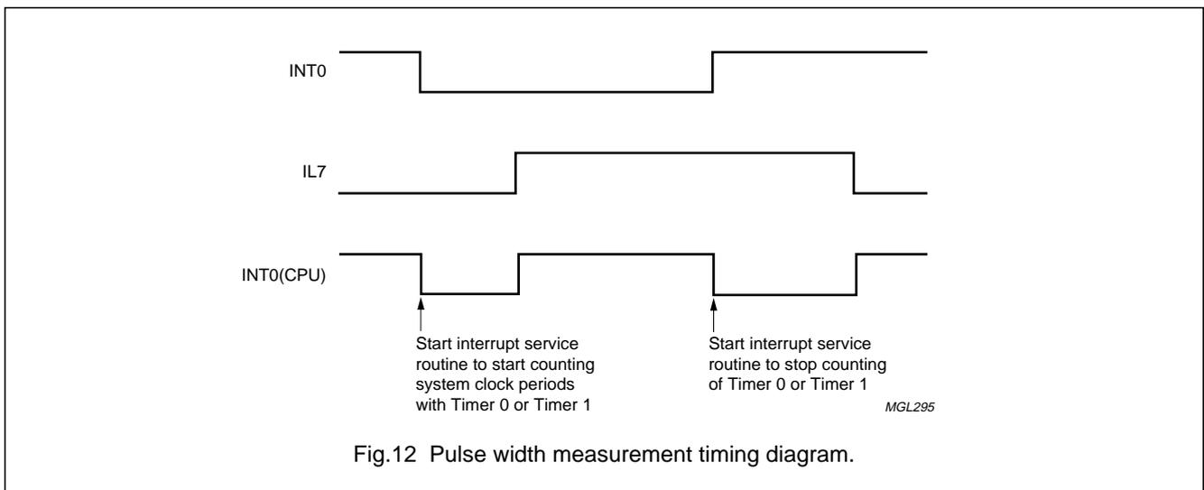
Fig.12 Pulse width measurement timing diagram.
