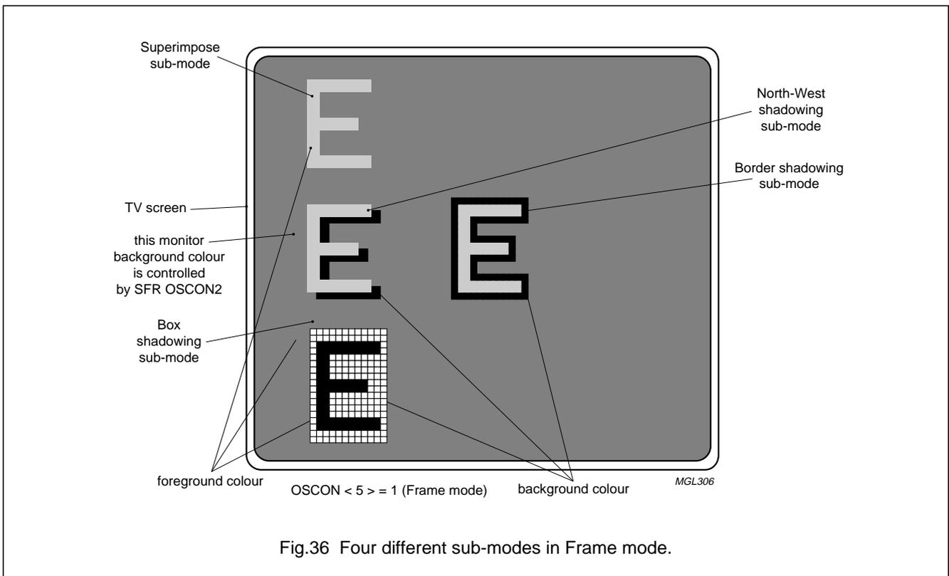
Fig.36 Four different sub-modes in Frame mode.
