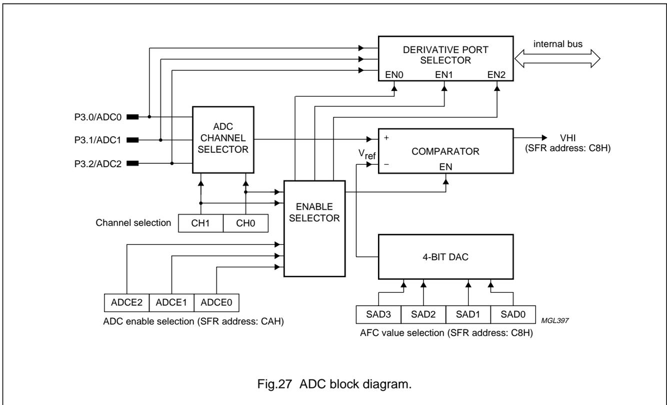
Fig.27 ADC block diagram.
