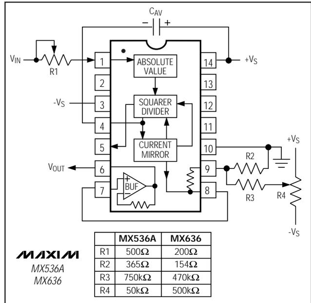
Figure 4. Optional External Gain and Output Offset Trims
