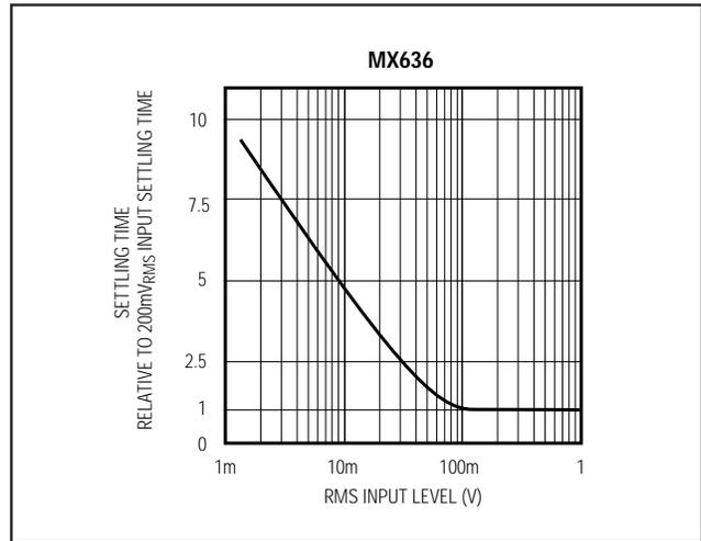
Figure 6b. MX636 Settling Time vs. Input Level
