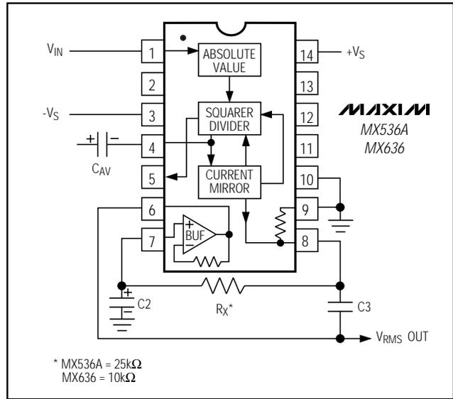
Figure 8. MX536A/MX636 with a Two-Pole Output Filter
