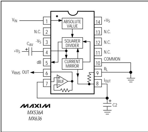
Figure 7. MX536A/MX636 with a One-Pole Output Filter
