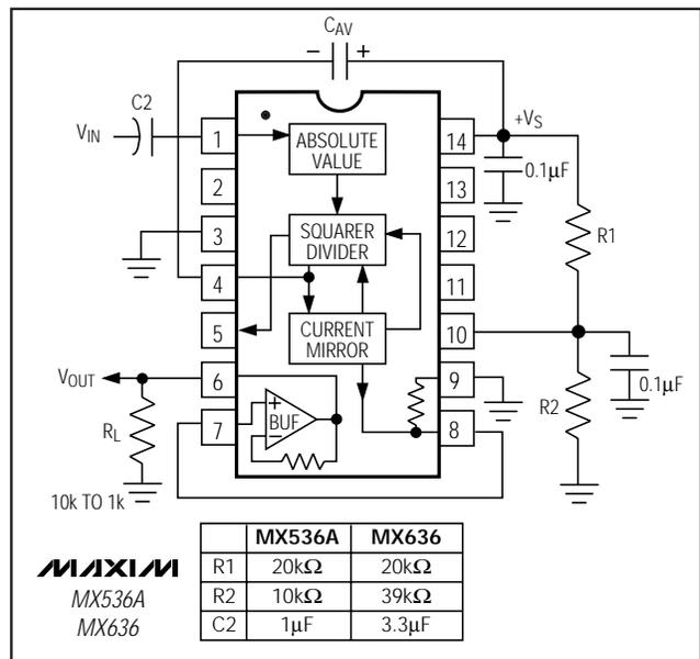
Figure 5. Single-Supply Operation
