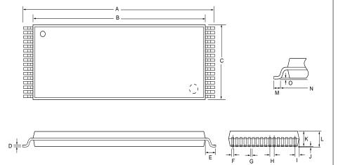
NOTE: Each lead certerline is located within .25mm[.01 inch] of its true position [TP] at a maximum at maximum material condition.
