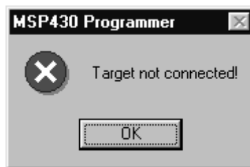
Figure 2–3. Communication Error Box for Blown Fuse
