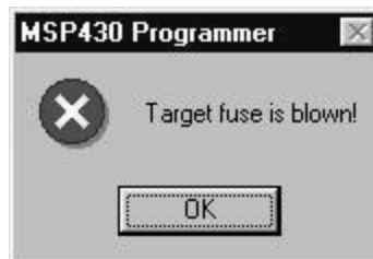
Figure 2–3. Communication Error Box for Blown Fuse
