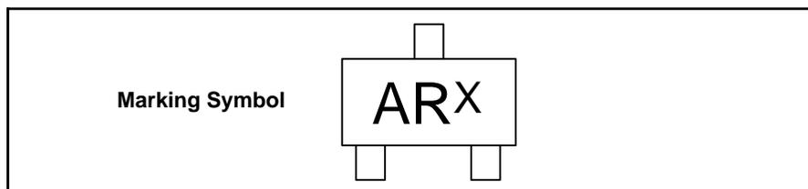
The "X" represents a smaller alpha digit Date Code. The Date Code indicates the actual month in which the part was manufactured.
