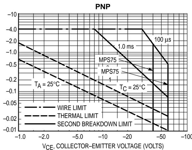
Figure 8. MPS750, MPS751 SOA,
