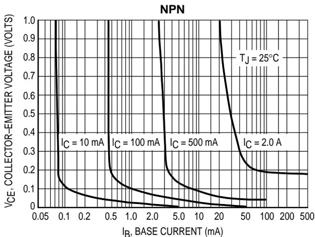
Figure 5. MPS650, MPS651
