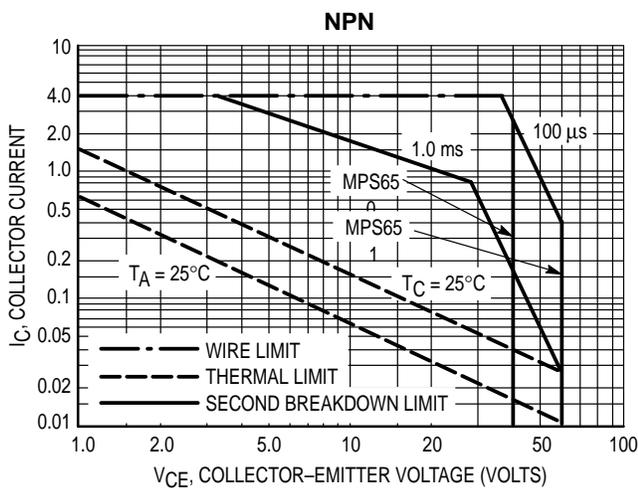
Figure 7. MPS650, MPS651 SOA,
