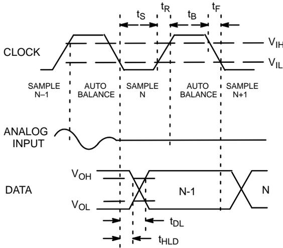
**Figure 1. MP7690A Timing Diagram**
