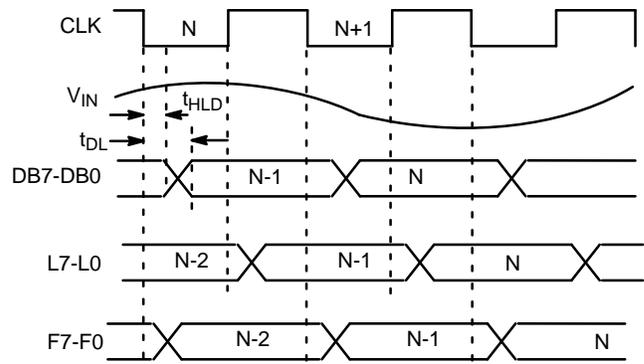
**Figure 10. MP7690A Functional Equivalent Circuit and Interface Timing**
