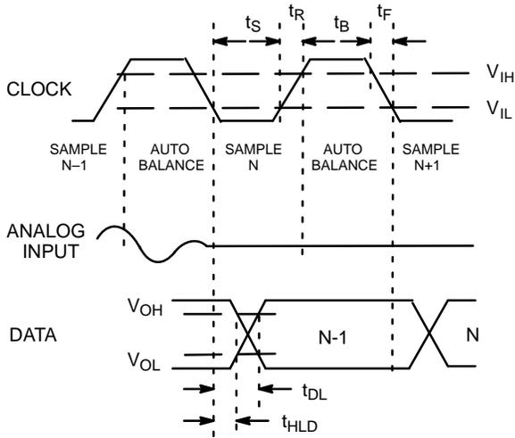
Figure 1. MP7684 Timing Diagram
