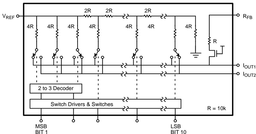
**3 Segment D/A Converter with Termination to GND.
