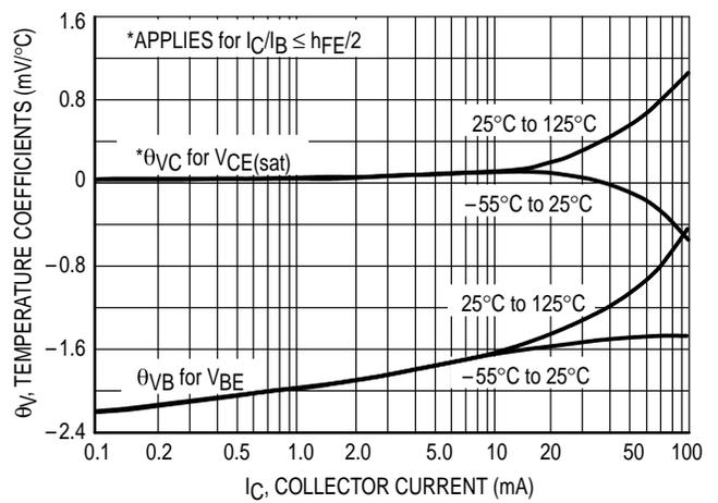
Figure 12. Temperature Coefficients
