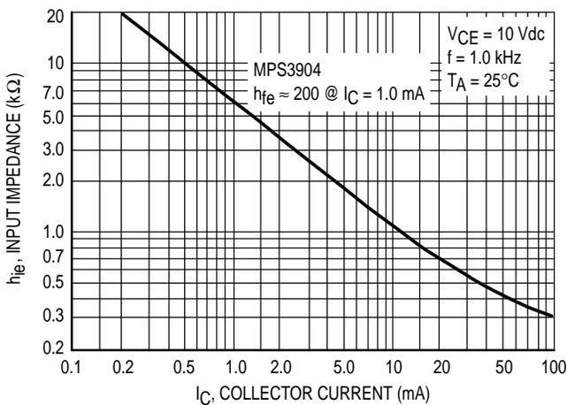
Figure 17. Input Impedance
