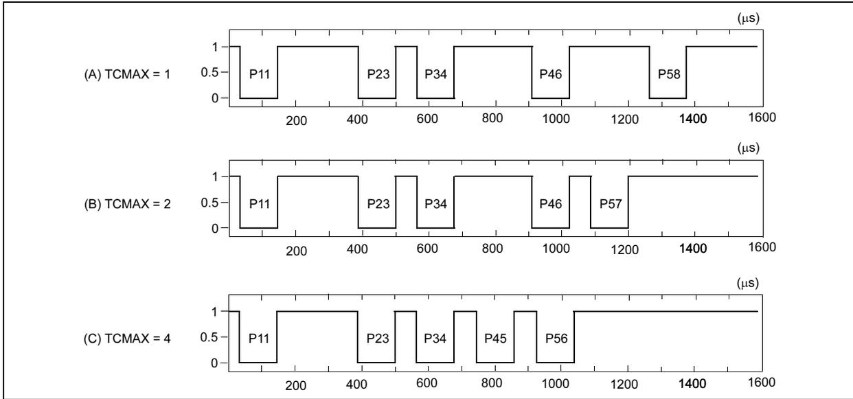
**FIGURE 6-7: GAP MODULATION PATTERNS FOR FRR, TSMAX = 64, TCMAX = 1**
