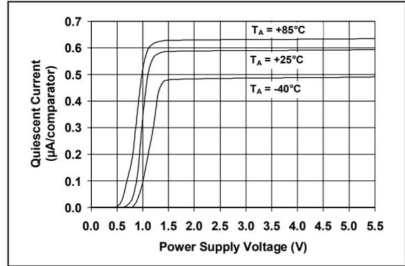
**FIGURE 2-16:** Quiescent Current vs. Power Supply Voltage.
