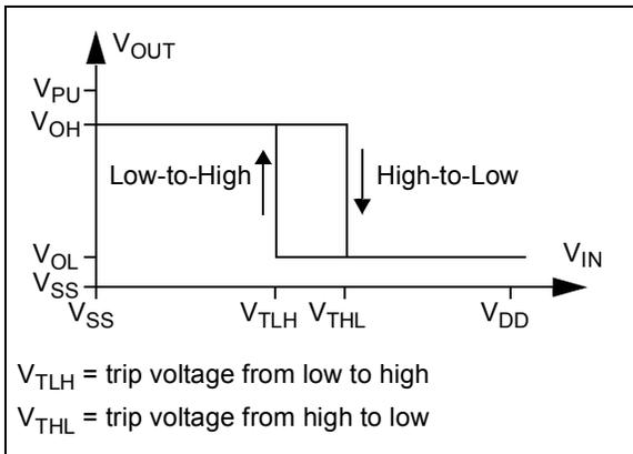
**FIGURE 3-4:** Hysteresis diagram for the inverting circuit.
