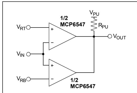
**FIGURE 3-8:** Windowed comparator.
