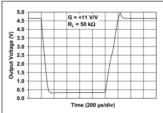
**FIGURE 2-31:** Large Signal Non-Inverting Pulse Response vs. Time.
