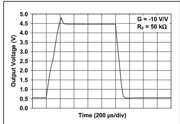
**FIGURE 2-34:** Large Signal Inverting Pulse Response vs. Time.
