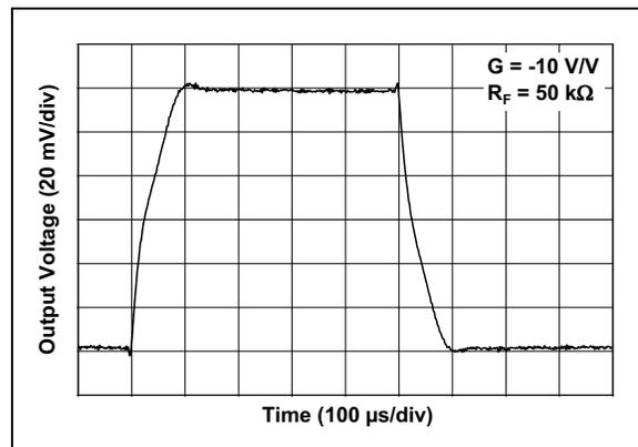
**FIGURE 2-30:** Small Signal Inverting Pulse Response vs. Time.
