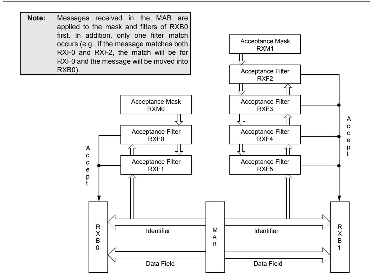
**FIGURE 4-3: RECEIVE FLOW FLOWCHART**
