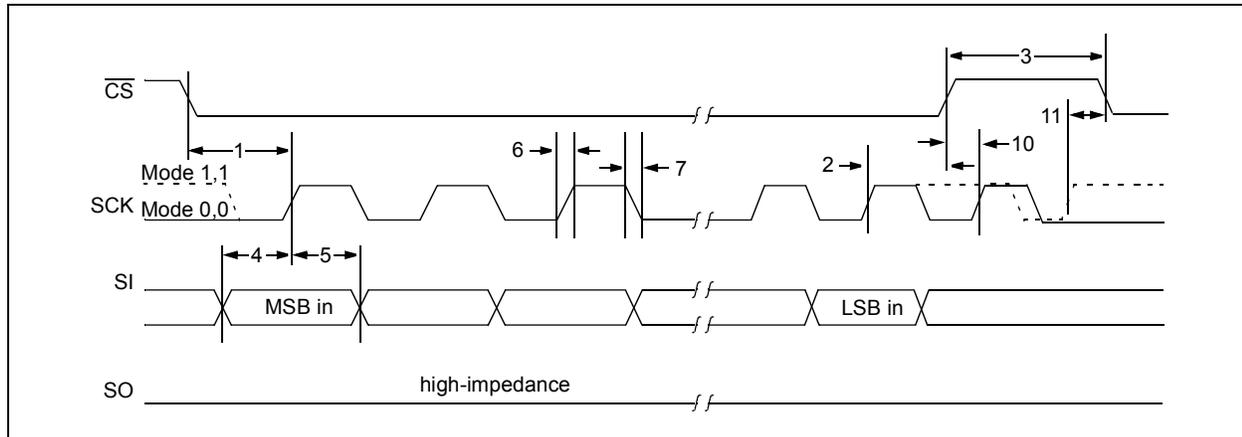
FIGURE 11-11: SPI™ OUTPUT TIMING
