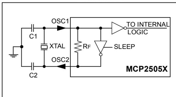
**FIGURE 8-2: EXTERNAL CLOCK INPUT OPERATION**
