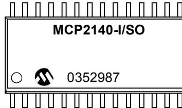
20-Lead SSOP (209 mil, 5.30 mm)
