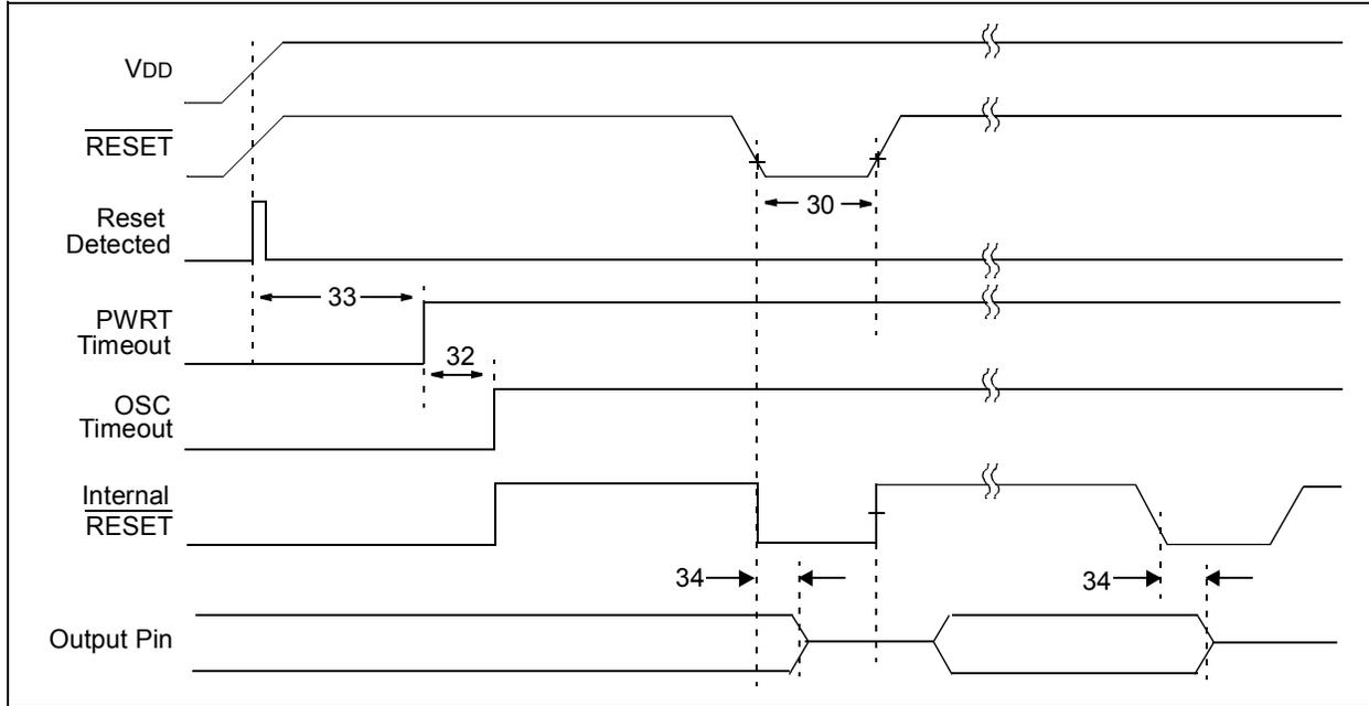
**TABLE 4-5:  $\overline{\text{RESET}}$  AND DEVICE RESET REQUIREMENTS**
