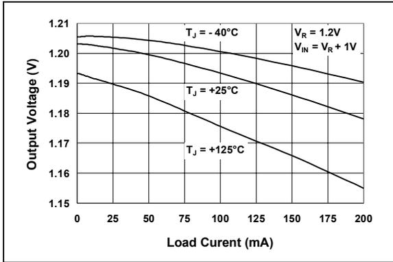
**FIGURE 2-8:** Output Voltage vs. Load Current ( $V_R = 1.2V$ ).
