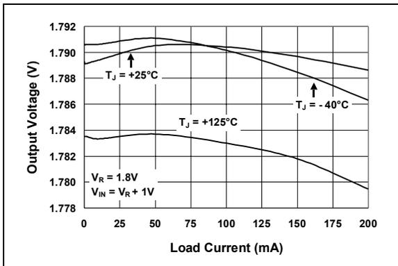
**FIGURE 2-9:** Output Voltage vs. Load Current ( $V_R = 1.8V$ ).
