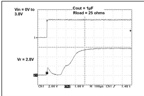
**FIGURE 2-26:** Start-up From  $V_{IN}$  ( $V_R = 2.8V$ ).
