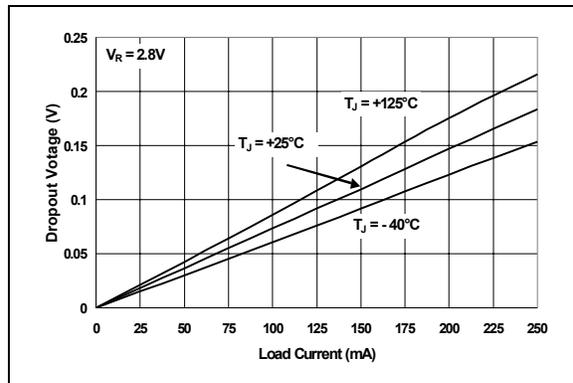
**FIGURE 2-12:** Dropout Voltage vs. Load Current ( $V_R = 2.8V$ ).
