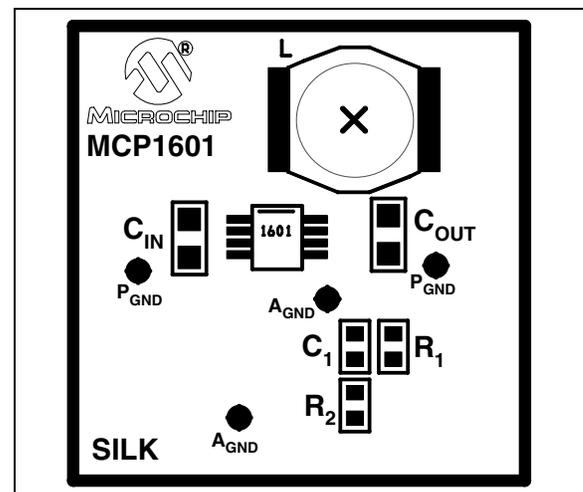
**FIGURE 5-2:** Component Placement.
