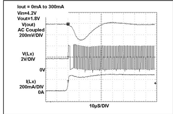
**FIGURE 2-16:** Load Step Response (PFM to PWM).
