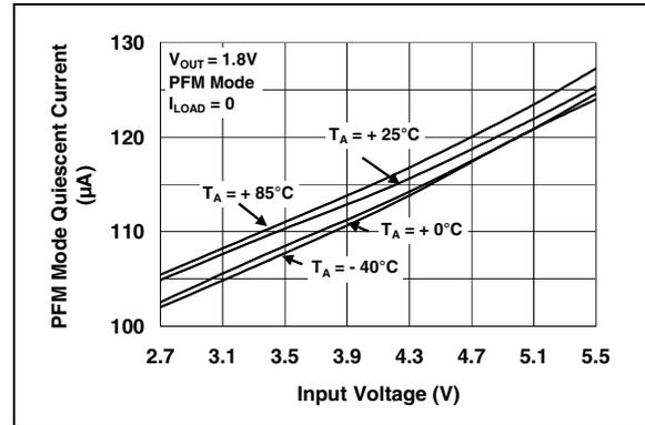
**FIGURE 2-4:** PFM Mode Quiescent Current vs. Input Voltage.
