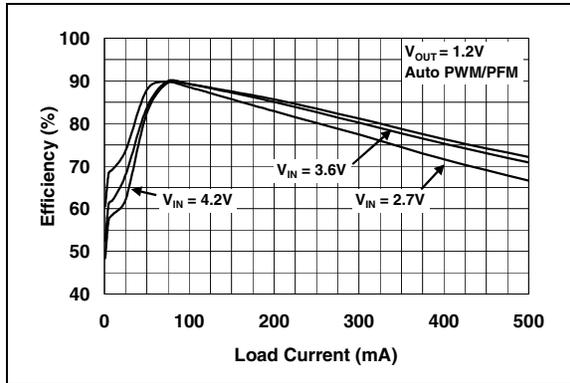
**FIGURE 2-1:** Efficiency vs. Load Current ( $V_{OUT} = 1.2V$ ).
