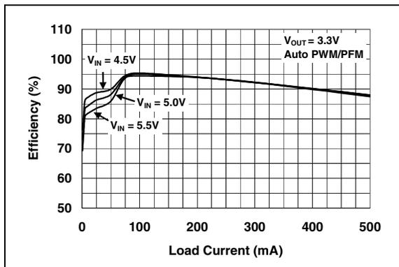
**FIGURE 2-3:** Efficiency vs. Load Current ( $V_{OUT} = 3.3V$ ).
