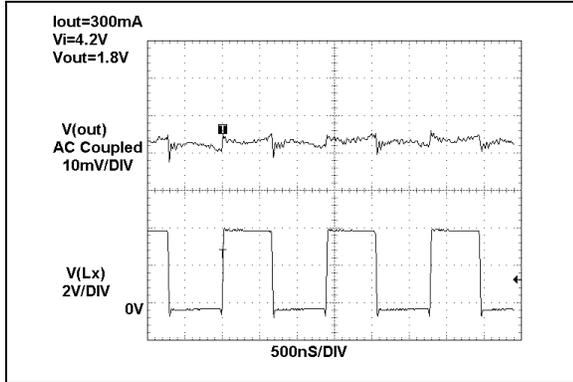
**FIGURE 2-19:** Typical Output Ripple Voltage (Forced PWM Mode).
