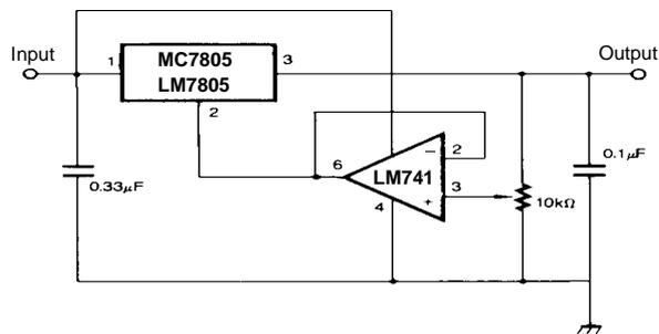
Figure 11. Adjustable Output Regulator (7 to 30V)
