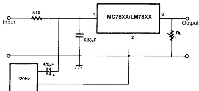
Figure 7. Ripple Rejection
