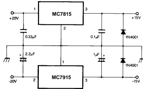
Figure 15. Split Power Supply (±15V-1A)
