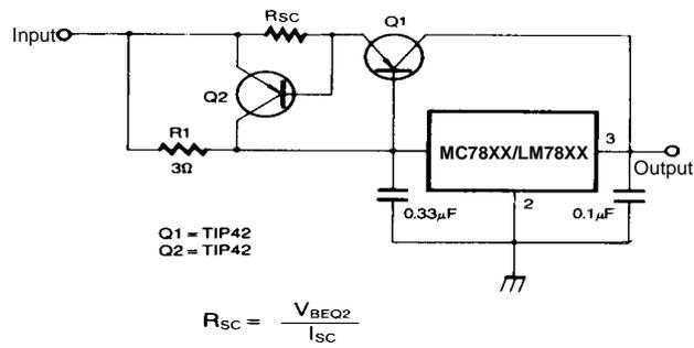
Figure 13. High Output Current with Short Circuit Protection
