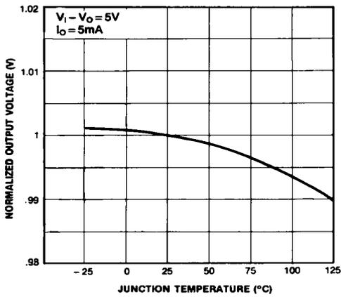
Figure 3. Output Voltage
