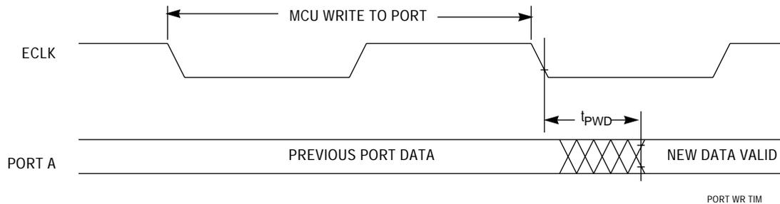
**Figure 71 Port Write Timing Diagram**
