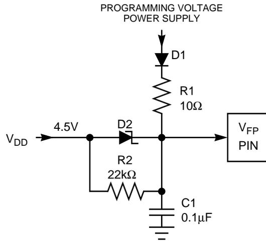
Figure 63 V<sub>FP</sub> Conditioning Circuit
