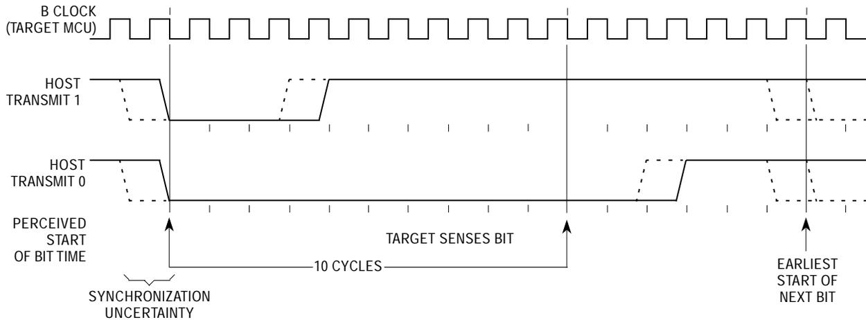
**Figure 60 BDM Host to Target Serial Bit Timing**
