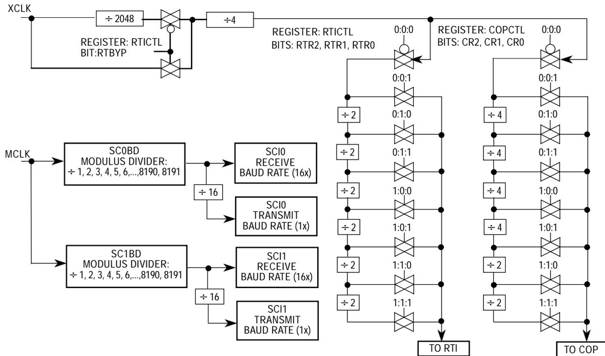
**Figure 19 Clock Chain for SCI0, SCI1, RTI, COP**
