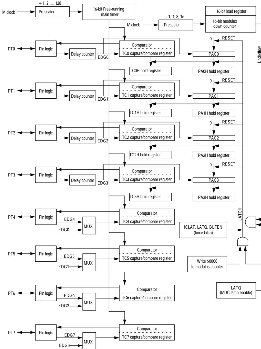
Figure 26 Timer Block Diagram in Latch Mode
