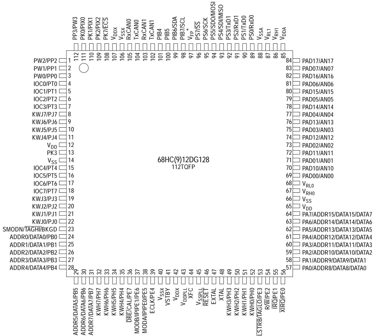
**Figure 2 Pin Assignments in 112-pin QFP for 68HC(9)12DG128**
