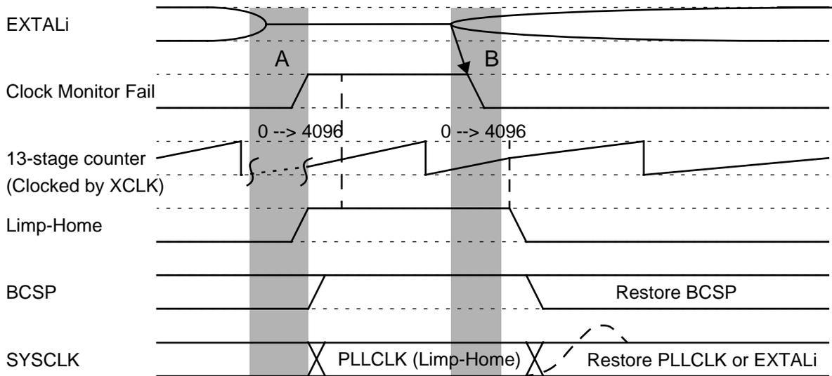
**Figure 15 Clock Loss during Normal Operation**
