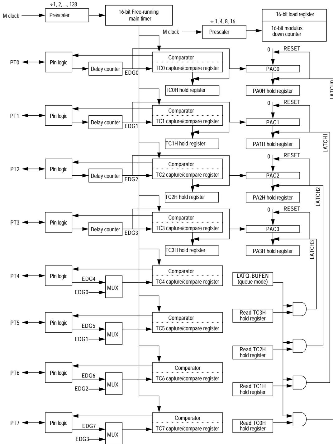
**Figure 27 Timer Block Diagram in Queue Mode**
