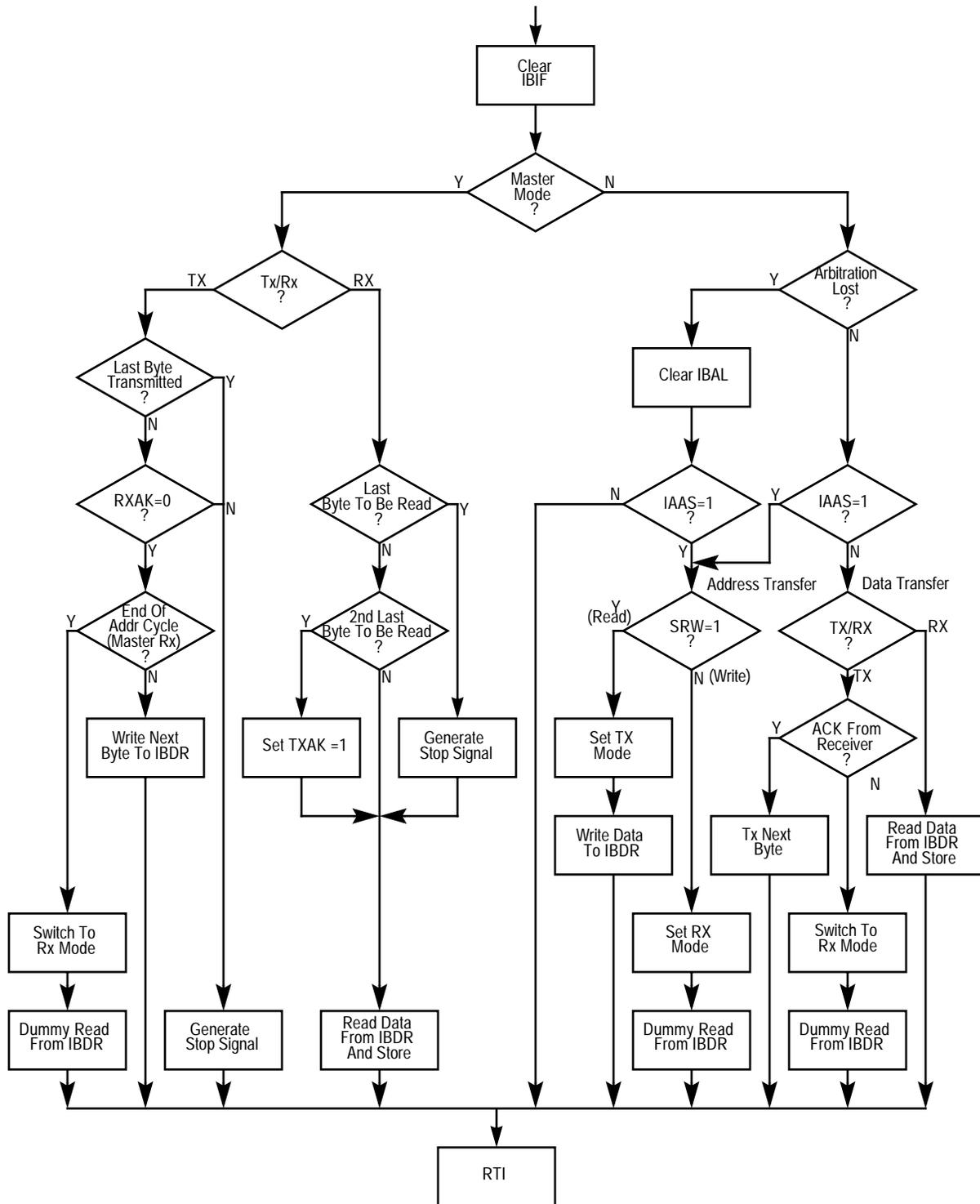
Figure 41 Flow-Chart of Typical IIC Interrupt Routine
