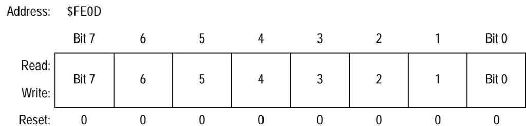
**Figure 20-5. Break Address Register Low (BRKL)**
