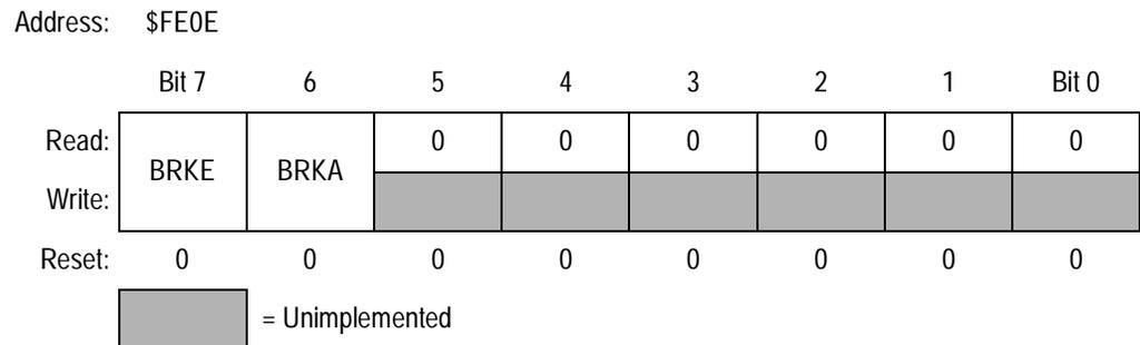
**Figure 20-3. Break Status and Control Register (BRKSCR)**
