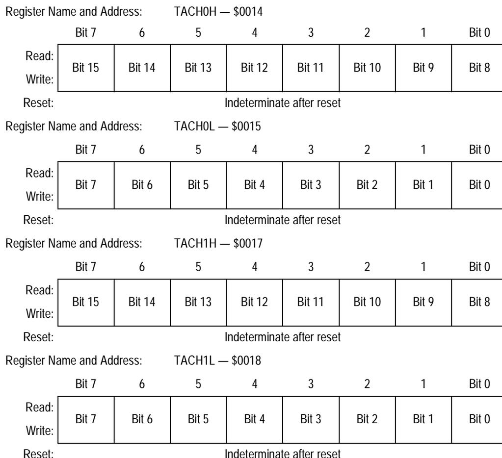
**Figure 11-9. TIMA Channel Registers
