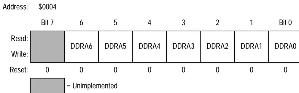
**Figure 14-3. Data Direction Register A (DDRA)**
