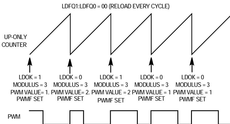
**Figure 9-9. Edge-Aligned PWM Value Loading**
