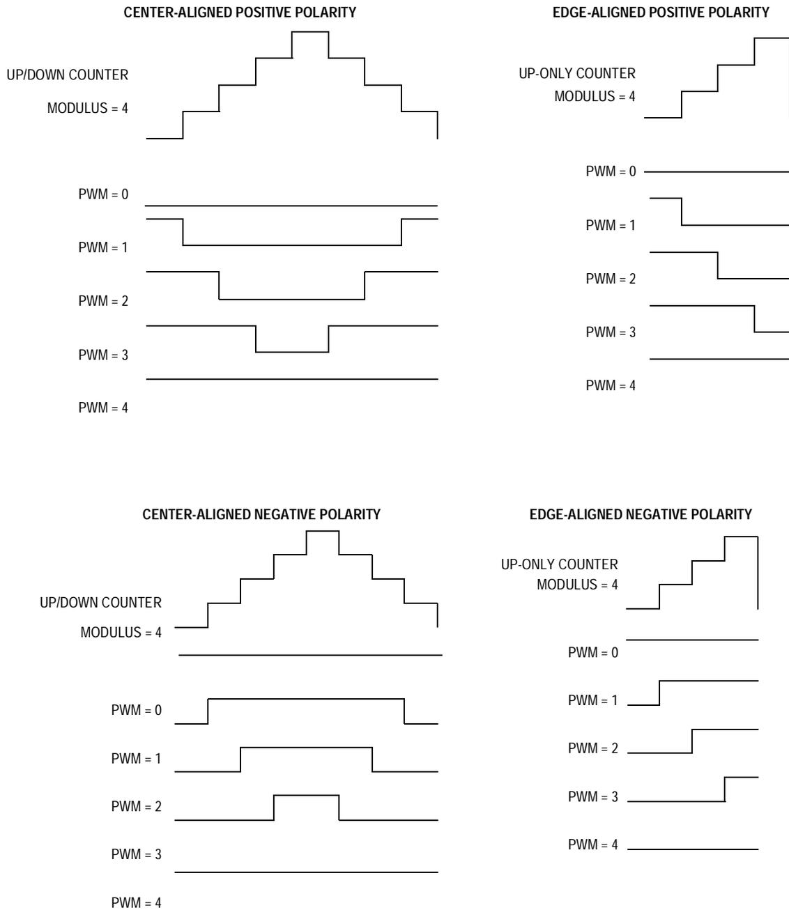
**Figure 9-17. PWM Polarity**
