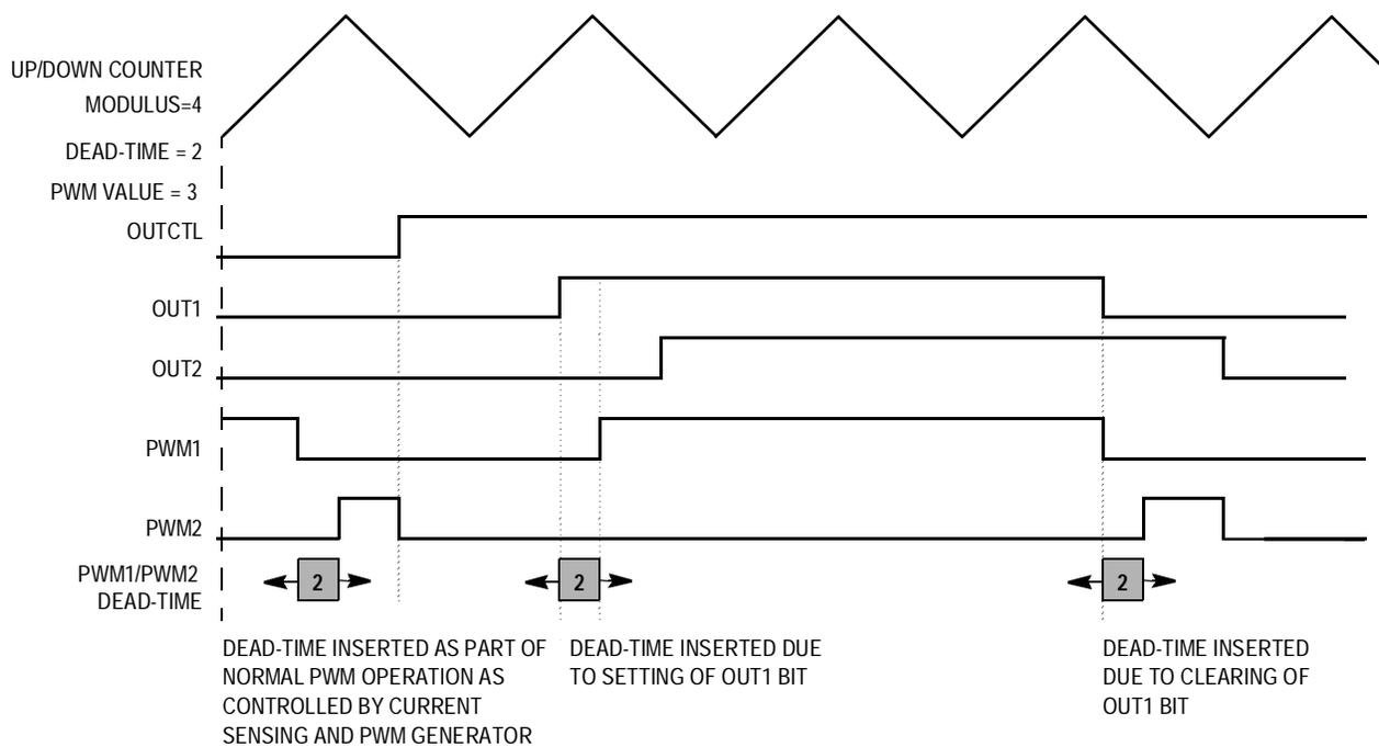
**Figure 9-19. Dead-Time Insertion During OUTCTL = 1**
