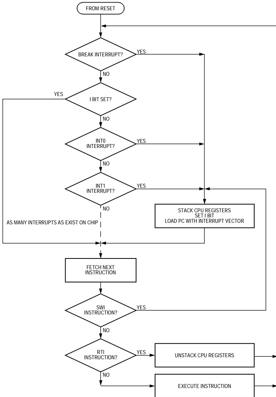
**Figure 7-9. Interrupt Processing**
