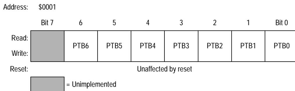
**Figure 14-5. Port B Data Register (PTB)**
