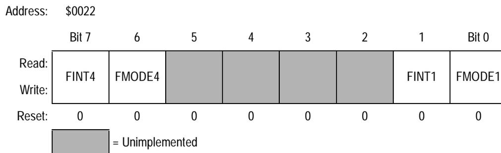
**Figure 9-39. Fault Control Register (FCR)**
