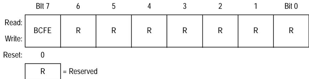
**Figure 7-17. SIM Break Flag Control Register (SBFCR)**
