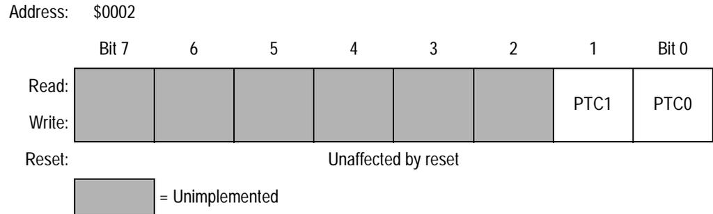
**Figure 14-8. Port C Data Register (PTC)**
