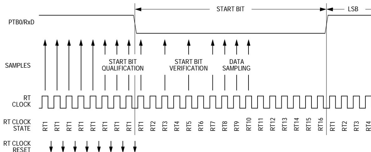
**Figure 13-6. Receiver Data Sampling**
