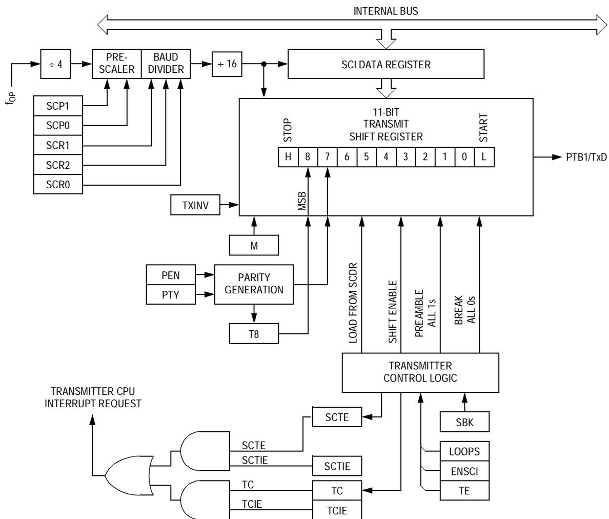
**Figure 13-4. SCI Transmitter**
