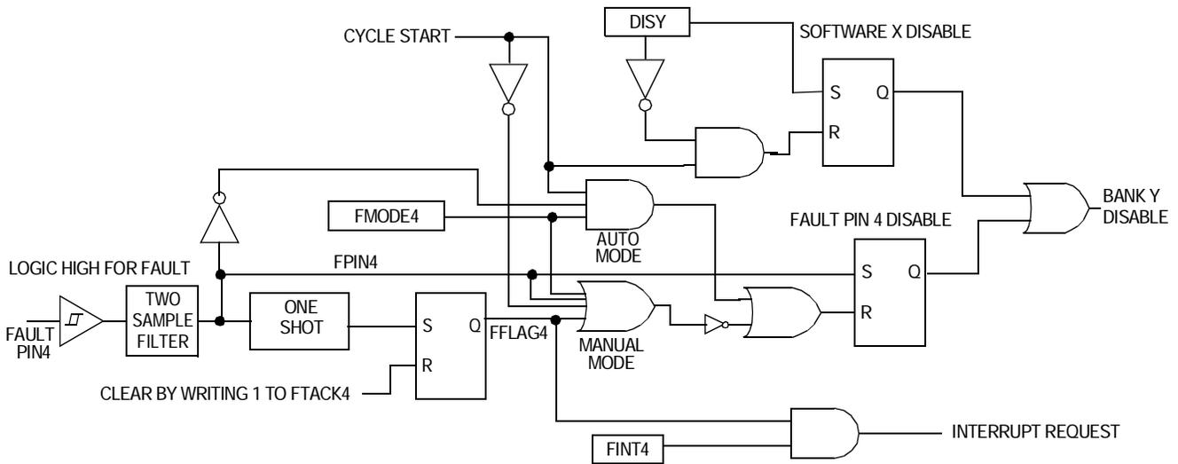
The example is of fault pin 4 with DISY.
