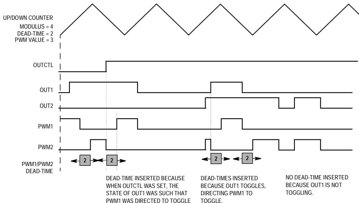
**Figure 9-20. Dead-Time Insertion During OUTCTL = 1**
