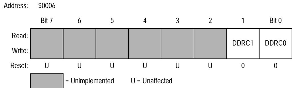
**Figure 14-9. Data Direction Register C (DDRC)**
