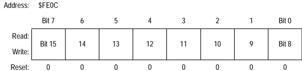
**Figure 20-4. Break Address Register High (BRKH)**
