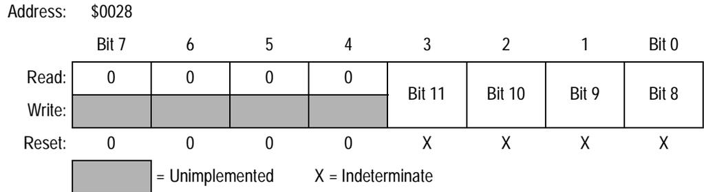
**Figure 9-31. PWM Counter Modulo Register High (PDMODH)**
