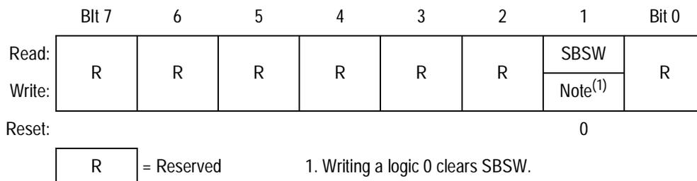
**Figure 7-15. SIM Break Status Register (SBSR)**
