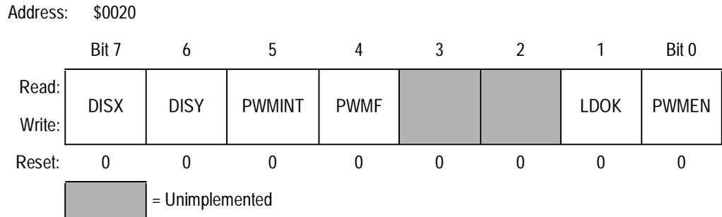
**Figure 9-35. PWM Control Register 1 (PCTL1)**
