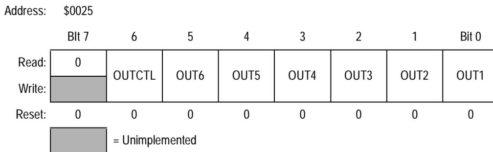
**Figure 9-18. PWM Output Control Register (PWMOUT)**
