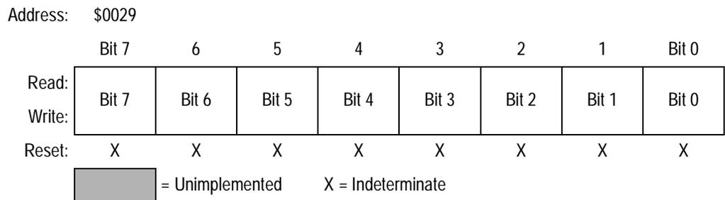
**Figure 9-32. PWM Counter Modulo Register Low (PDMODL)**
