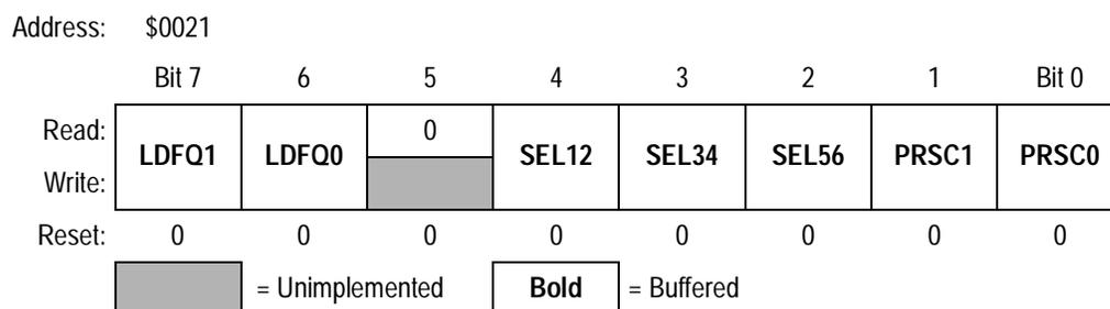
**Figure 9-36. PWM Control Register 2 (PCTL2)**
