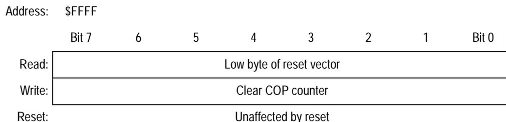
**Figure 15-3. COP Control Register (COPCTL)**
