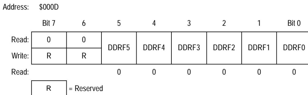
**Figure 15-17. Data Direction Register F (DDRF)**
