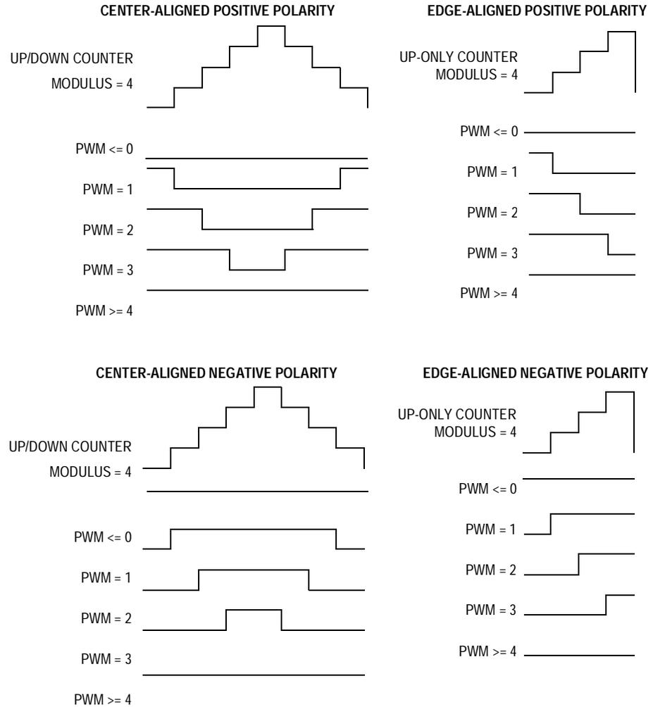
**Figure 9-20. PWM Polarity**
