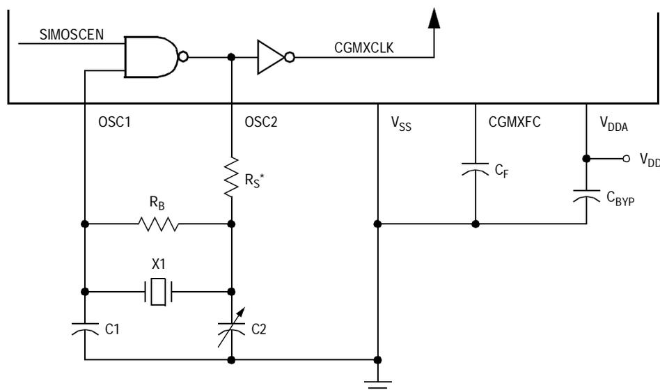
\* $R_S$  can be 0 (shorted) when used with higher-frequency crystals. Refer to manufacturer's data.
