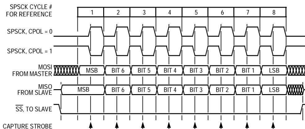
**Figure 13-4. Transmission Format ( $CPHA = 0$ )**
