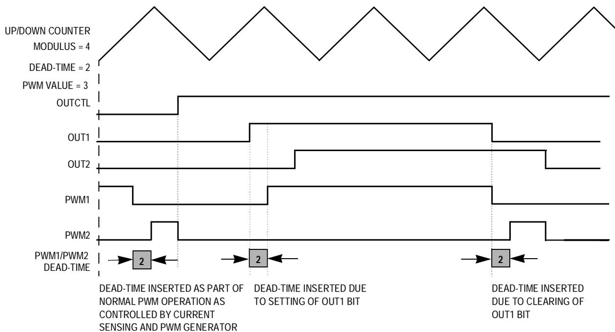
**Figure 9-22. Dead-Time Insertion During OUTCTL = 1**
