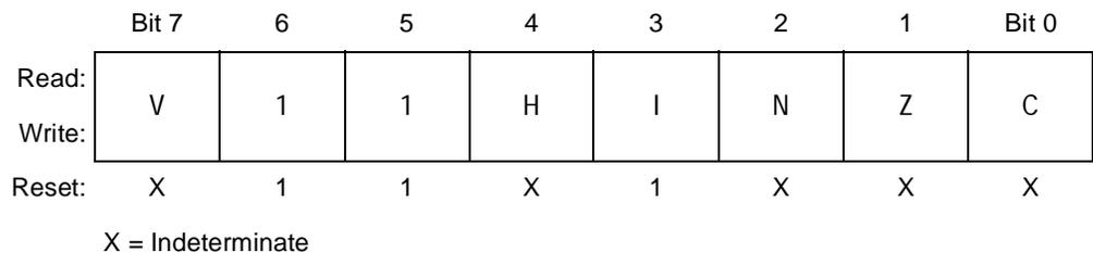
**Figure 6-6. Condition Code Register (CCR)**
