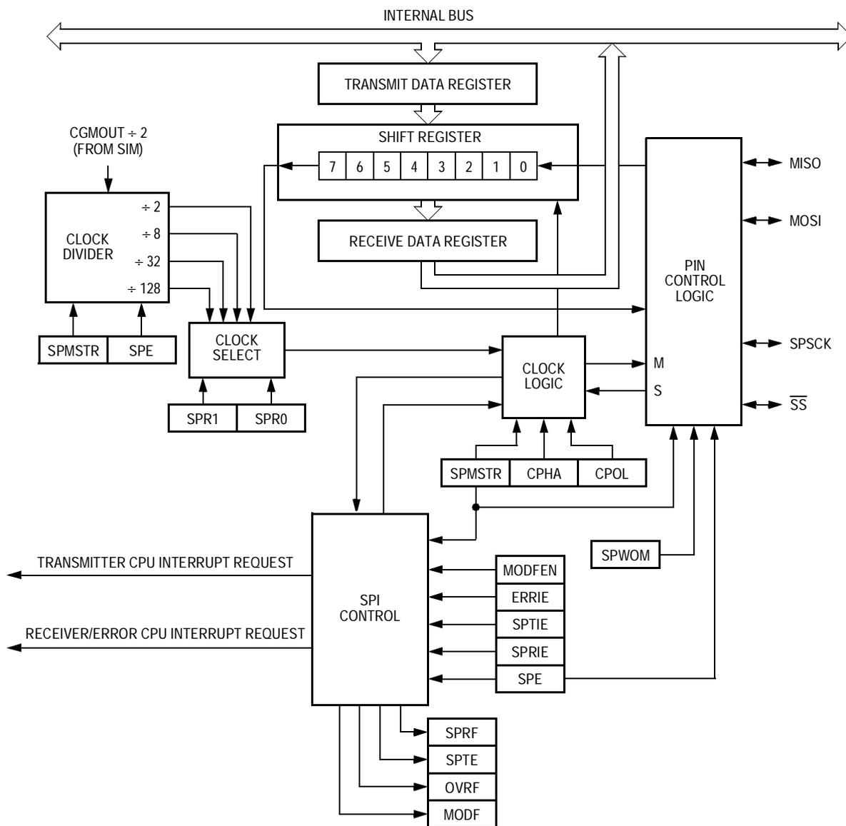
**Figure 13-1. SPI Module Block Diagram**
