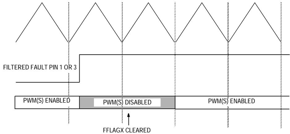
**Figure 9-28. PWM Disabling in Manual Mode (Example 1)**
