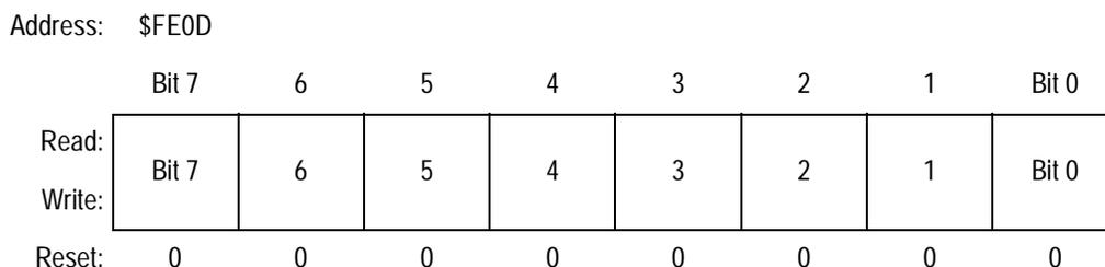
**Figure 21-5. Break Address Register Low (BRKL)**
