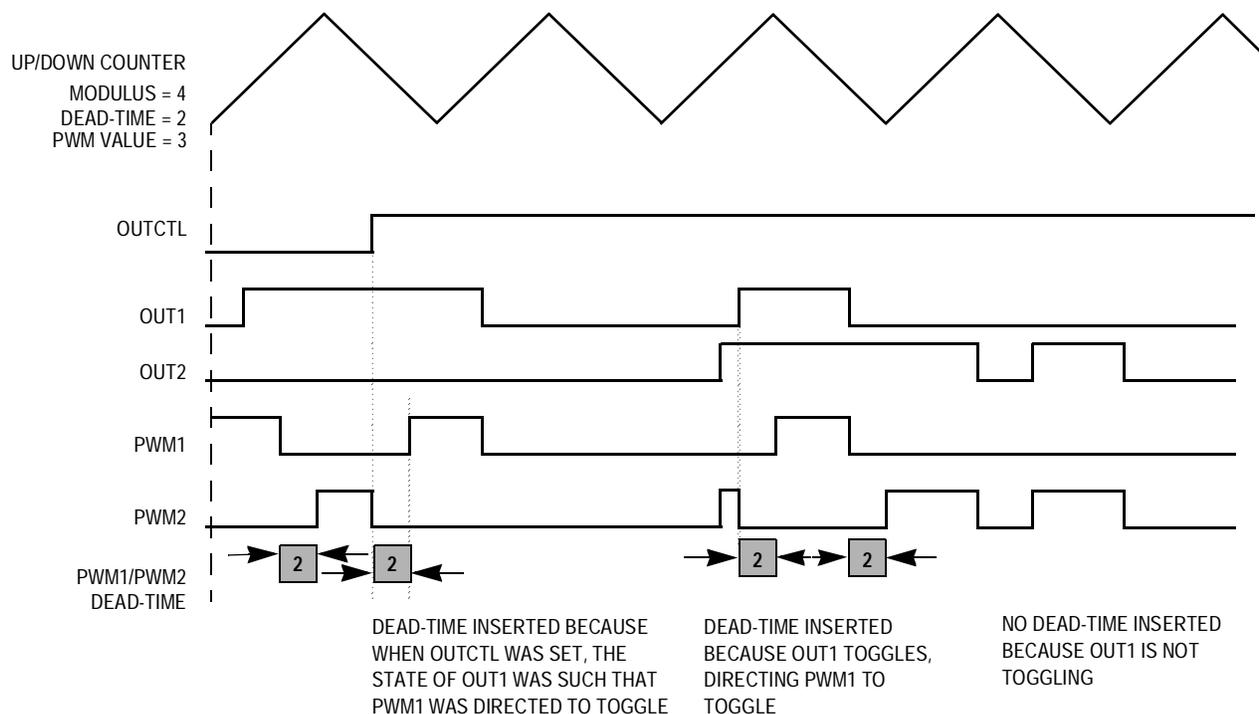
**Figure 9-23. Dead-Time Insertion During OUTCTL = 1**
