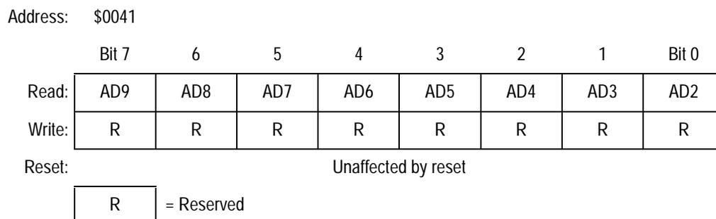
**Figure 19-4. ADC Data Register High (ADRH)
