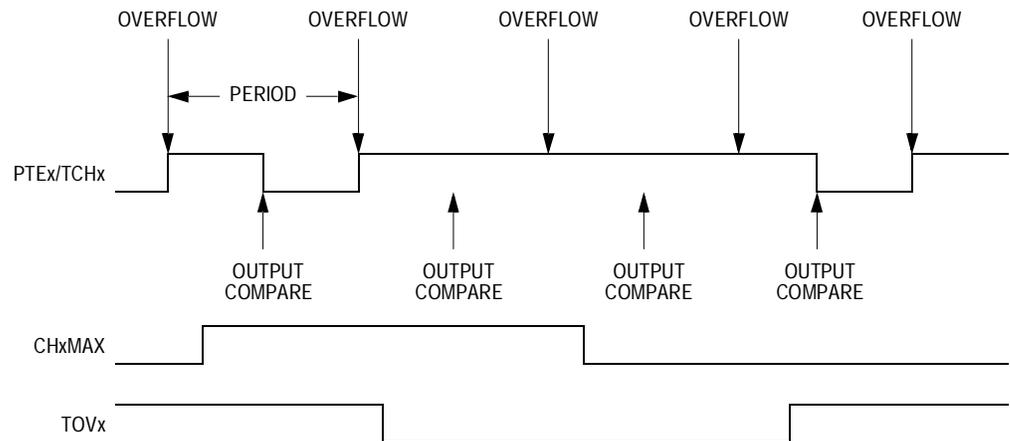
**Figure 11-8. CH<sub>x</sub>MAX Latency**
