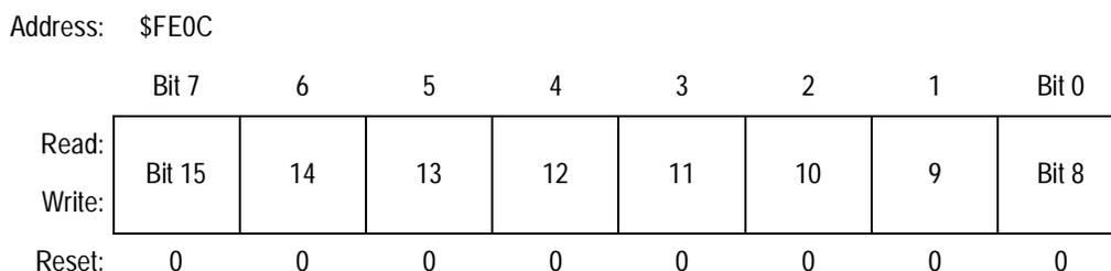
**Figure 21-4. Break Address Register High (BRKH)**
