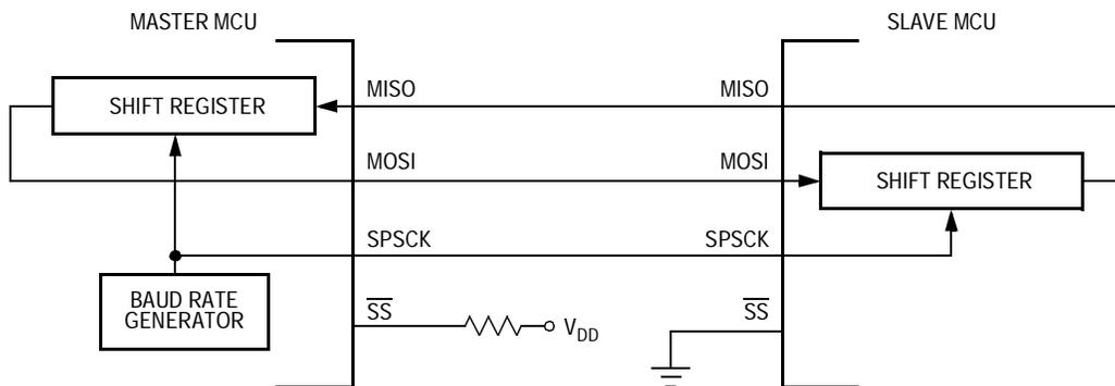
**Figure 13-3. Full-Duplex Master-Slave Connections**
