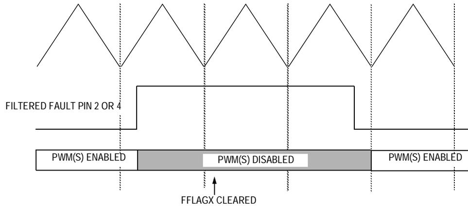
**Figure 9-29. PWM Disabling in Manual Mode (Example 2)**
