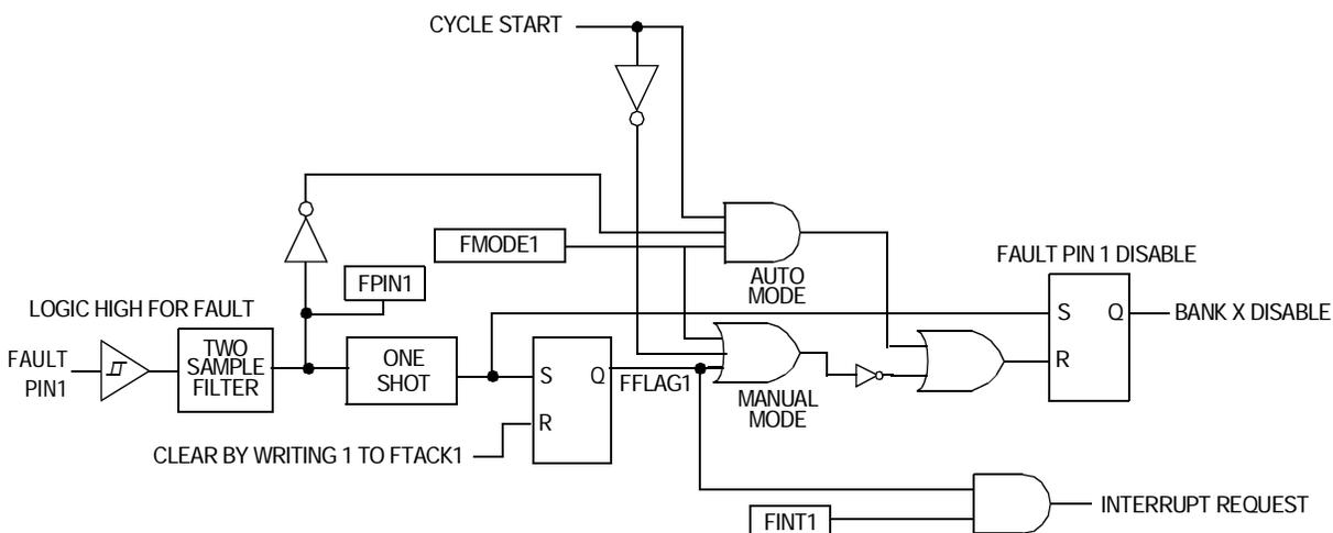
The example is of fault pin 1. Fault pin 3 is logically similar and affects BANK Y disable.
