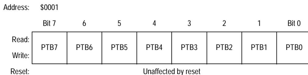
**Figure 15-5. Port B Data Register (PTB)**
