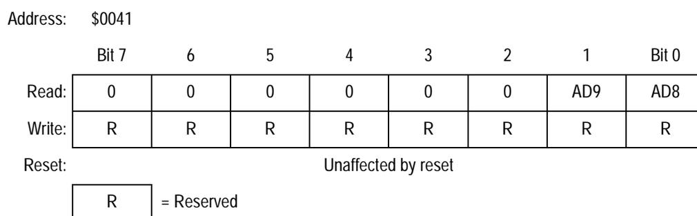
**Figure 19-5. ADC Data Register High (ADRH)
