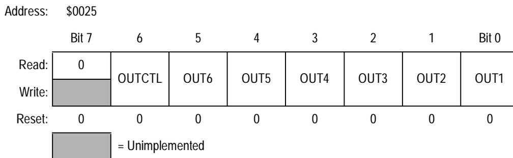
**Figure 9-21. PWM Output Control Register (PWMOUT)**
