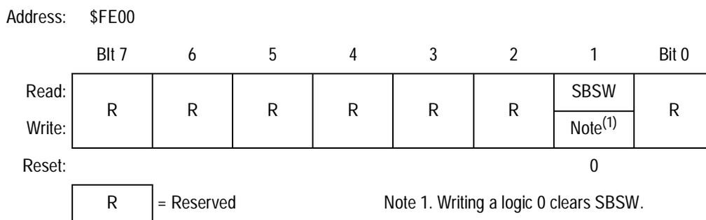
**Figure 7-14. SIM Break Status Register (SBSR)**
