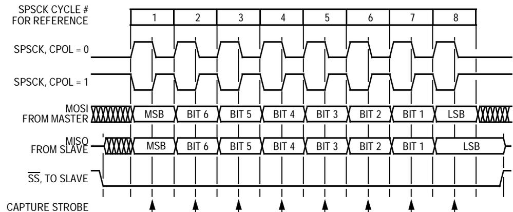
**Figure 13-6. Transmission Format ( $CPHA = 1$ )**
