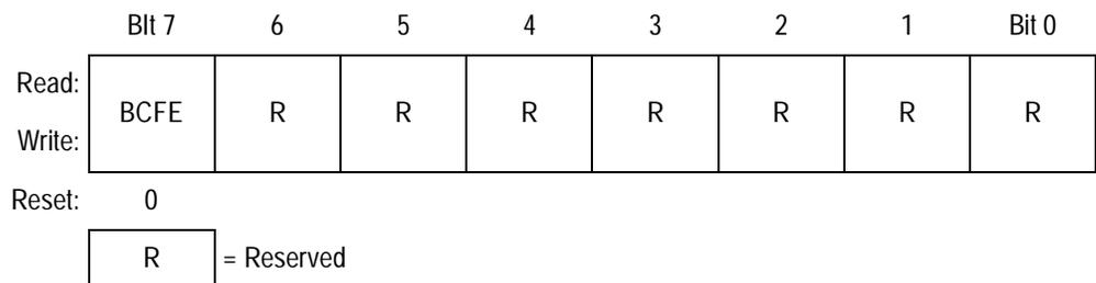
**Figure 7-16. SIM Break Flag Control Register (SBFCR)**
