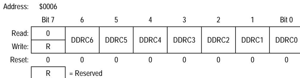
**Figure 15-9. Data Direction Register C (DDRC)**
