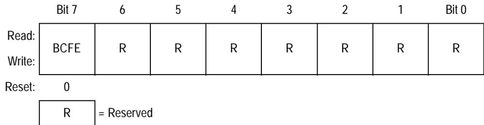
**Figure 21-7. SIM Break Flag Control Register (SBFCR)**
