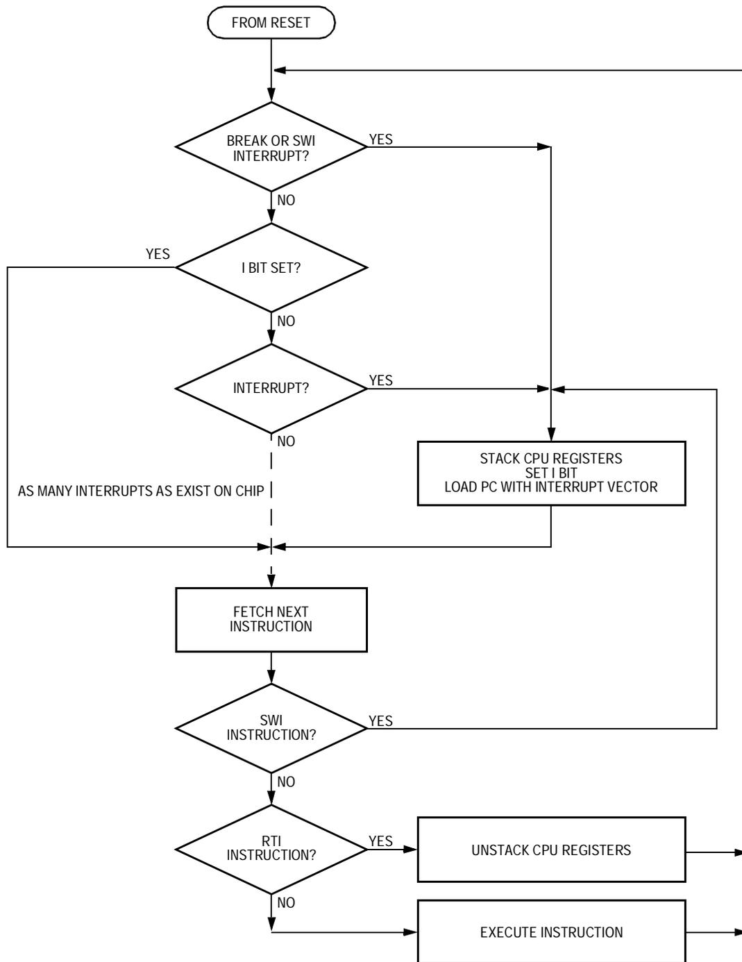
**Figure 7-8. Interrupt Processing**
