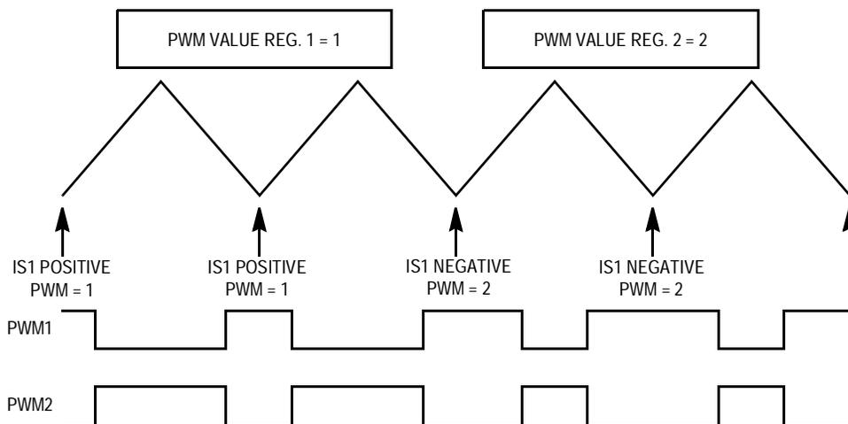
**Figure 9-19. Top/Bottom Correction for PWMs 1 and 2**
