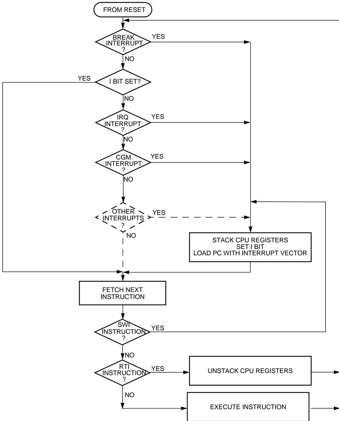
Figure 4-6. Interrupt Processing
