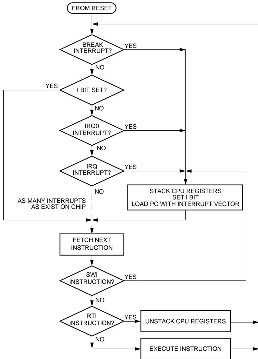
**Figure 19-10. Interrupt Processing**
