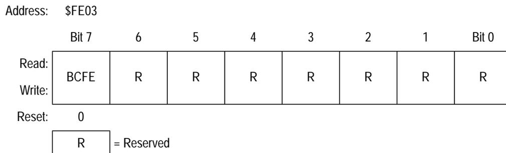
**Figure 6-7. SIM Break Flag Control Register (SBFCR)**
