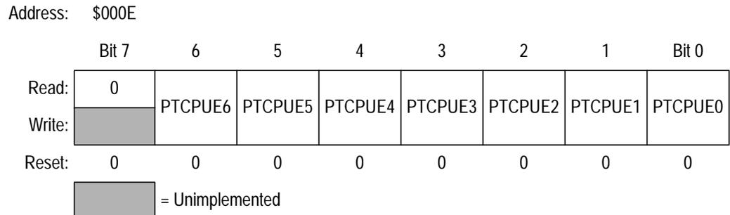
**Figure 16-12. Port C Input Pullup Enable Register (PTCPUE)**
