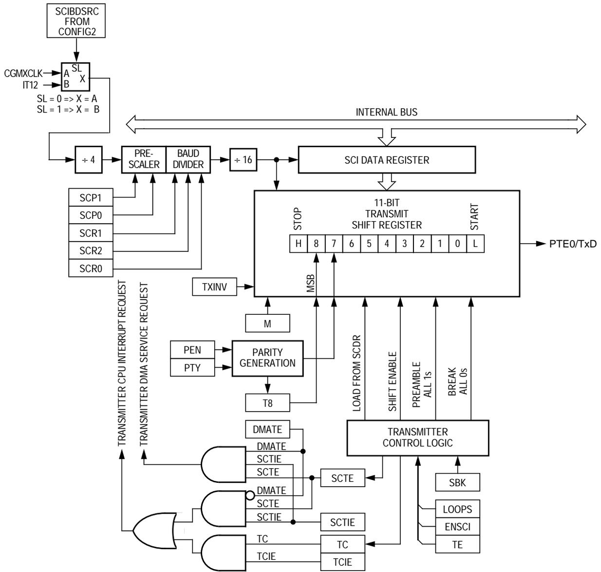
**Figure 18-4. SCI Transmitter**
