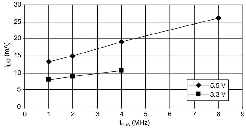
**Figure 23-7. Typical Operating I<sub>DD</sub> with All Modules Turned On (–40 °C to 85 °C)**
