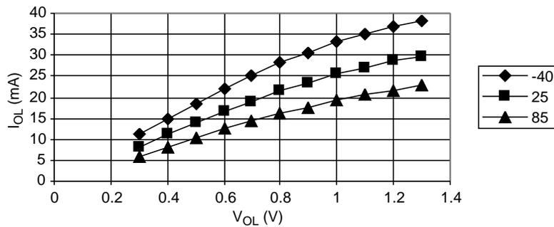
$V_{OL} < 0.8 \text{ V} @ I_{OL} = 10 \text{ mA}$
