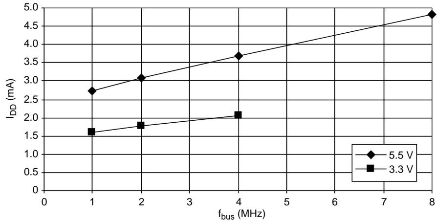
**Figure 23-8. Typical Wait Mode I<sub>DD</sub> with TBM Enabled, LVI Disabled, and PLL Disabled (–40 °C to 85 °C)**
