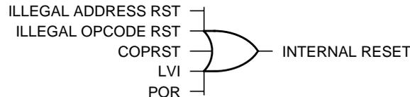
**Figure 19-6. Sources of Internal Reset**
