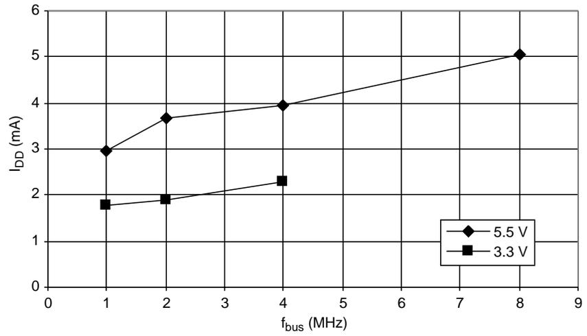
**Figure 23-9. Typical Wait Mode I<sub>DD</sub>, with LVI and TBM Enabled, PLL Disabled (–40 °C to 85 °C)**
