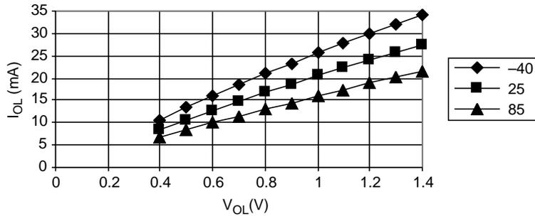
$V_{OL} < 0.4 \text{ V @ } I_{OL} = 1.6 \text{ mA}$
