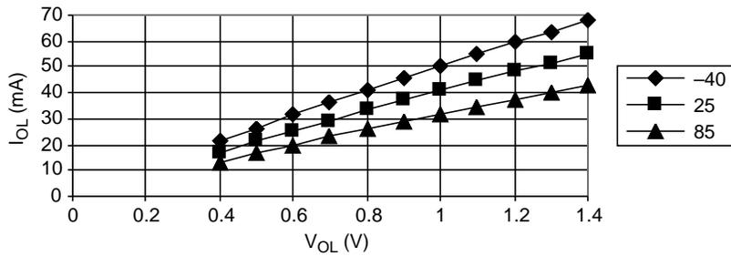
$V_{OL} < 1.0 \text{ V} @ I_{OL} = 15 \text{ mA}$
