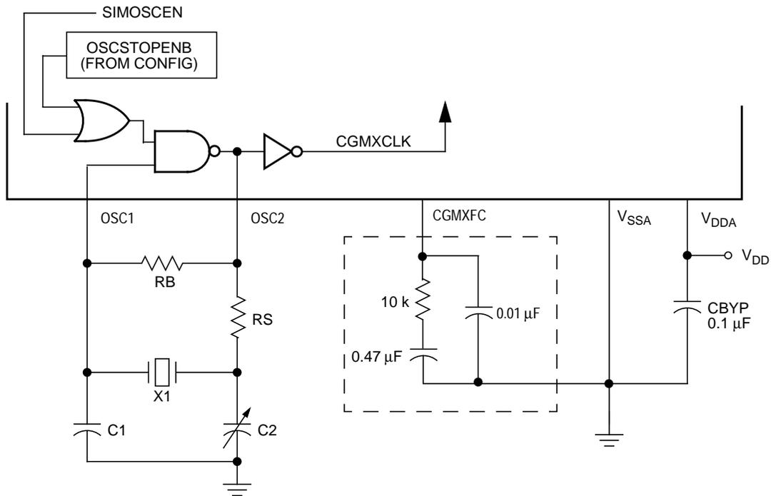
Note: Filter network in box can be replaced with a 0.47  $\mu\text{F}$  capacitor, but will degrade stability.
