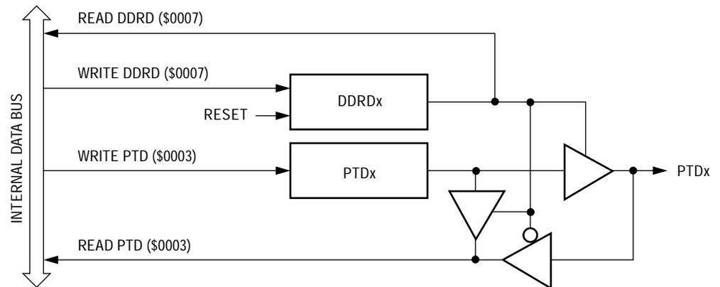
**Figure 13. Port D I/O Circuit**
