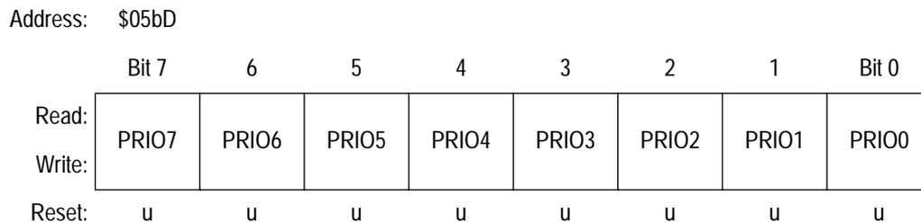
**Figure 13. Transmit Buffer Priority Register (TBPR)**
