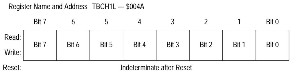
**Figure 9. TIMB Channel Registers
