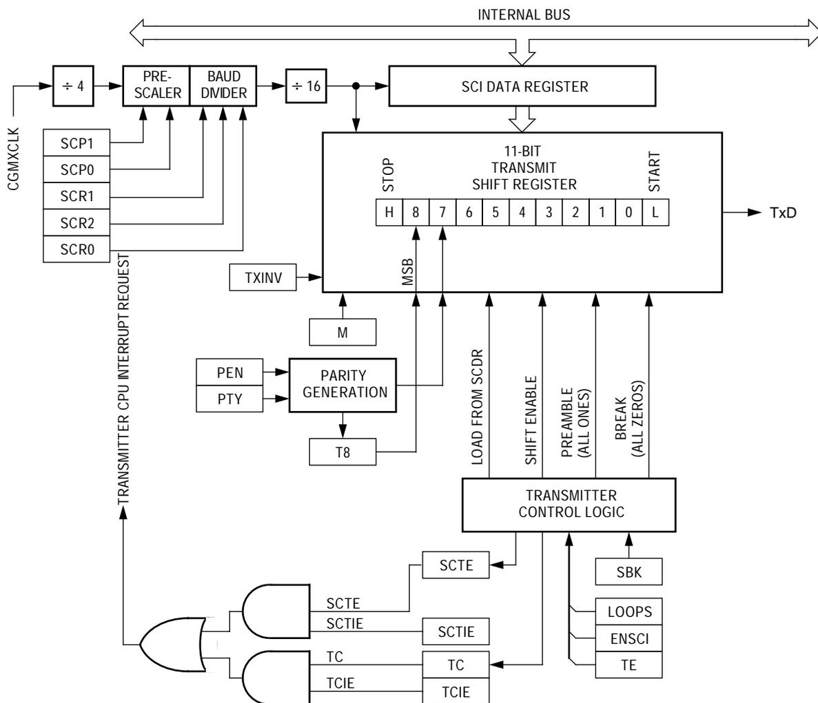
**Figure 4. SCI Transmitter**
