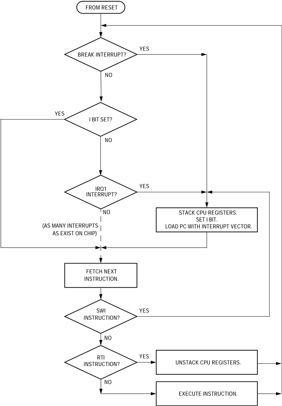
**Figure 9. Interrupt Processing**
