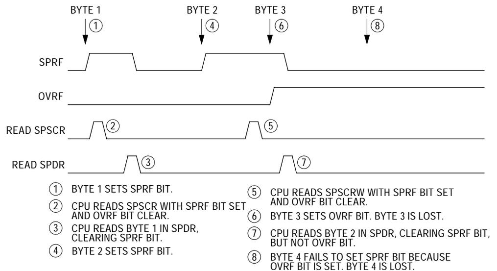
**Figure 6. Missed Read of Overflow Condition**
