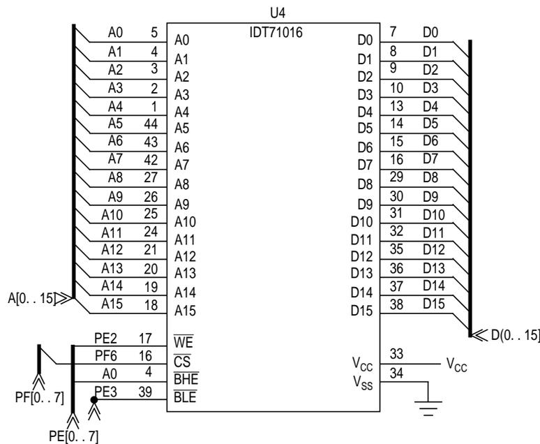
Figure 11-3. Expanded Wide Mode FLASH EEPROM Expansion Schematic (Sheet 2 of 3)
