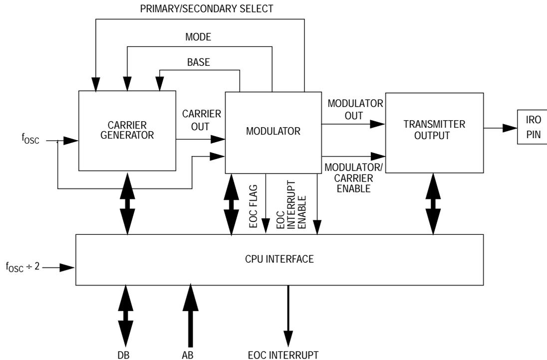
**Figure 9-1. Carrier Modulator Transmitter Module Block Diagram**
