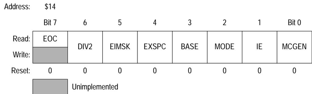
**Figure 9-10. Modulator Control and Status Register (MCSR)**
