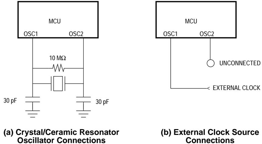
**Figure 1-5. Oscillator Connections**
