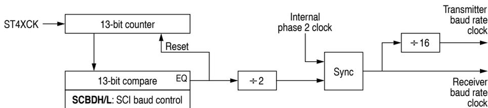
Figure 5-1 SCI baud rate generator circuit diagram
