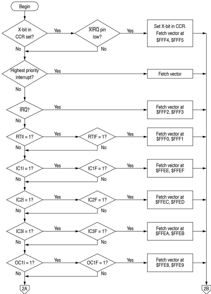
Figure 10-3 Interrupt priority resolution (1 of 3)
