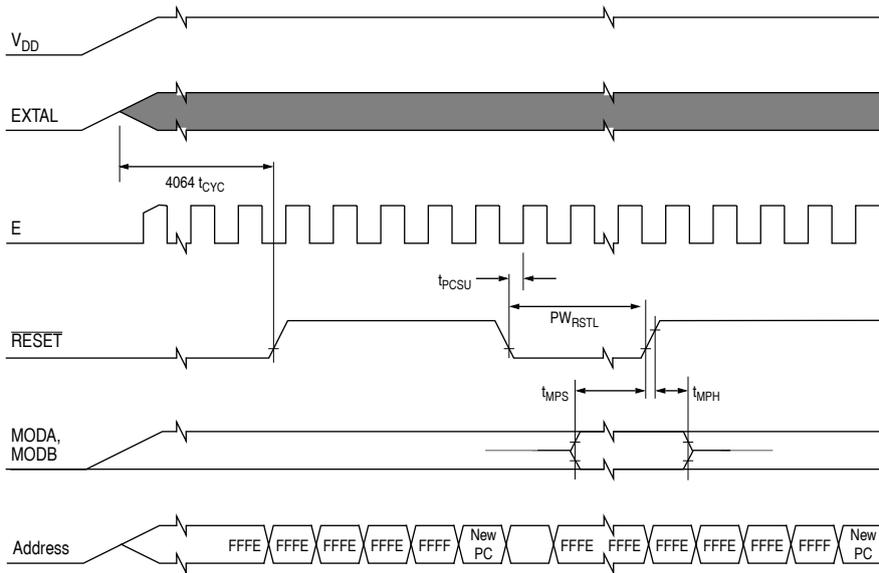
Figure 12-3 Reset timing
