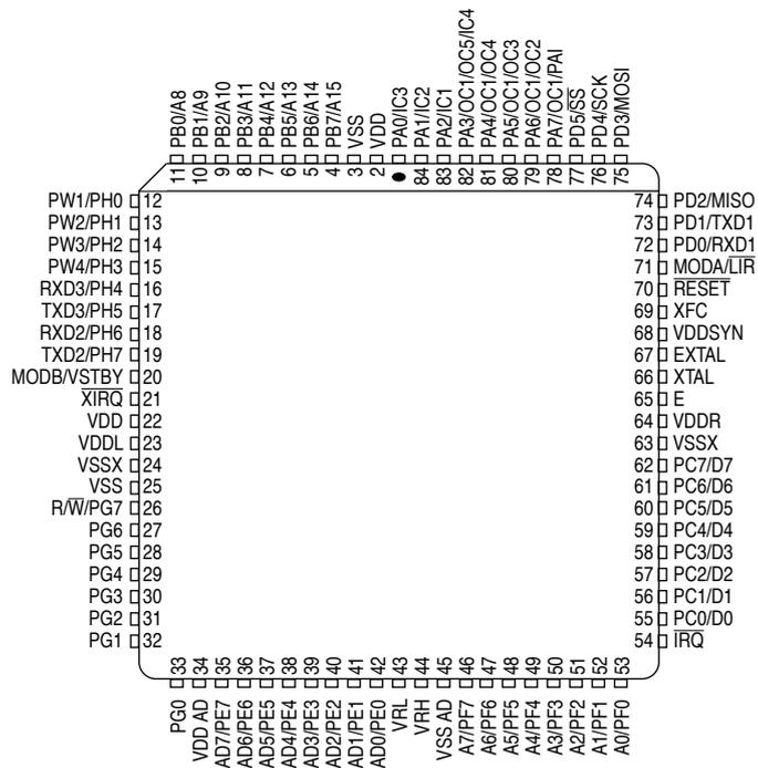
**Figure 2-1** 84-pin PLCC/CERQUAD pinout
