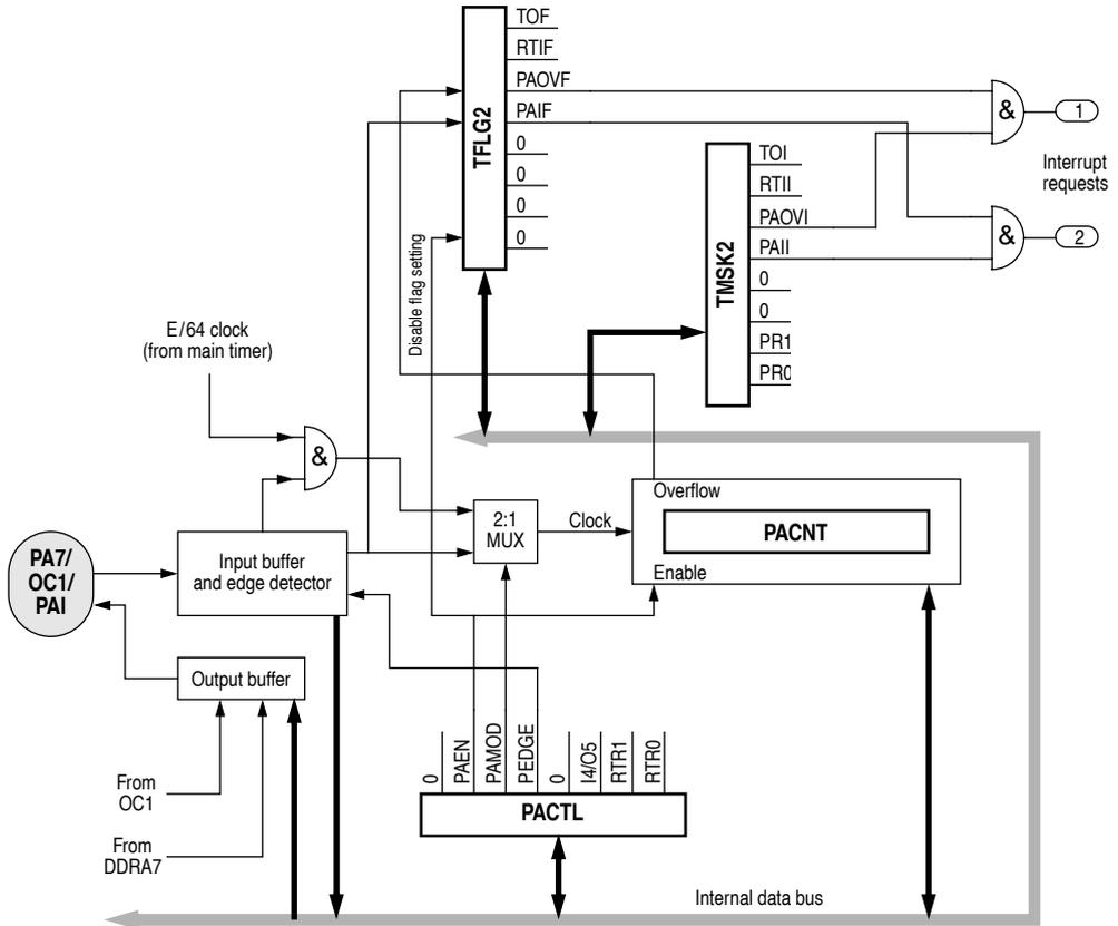
**Figure 8-3** Pulse accumulator block diagram
