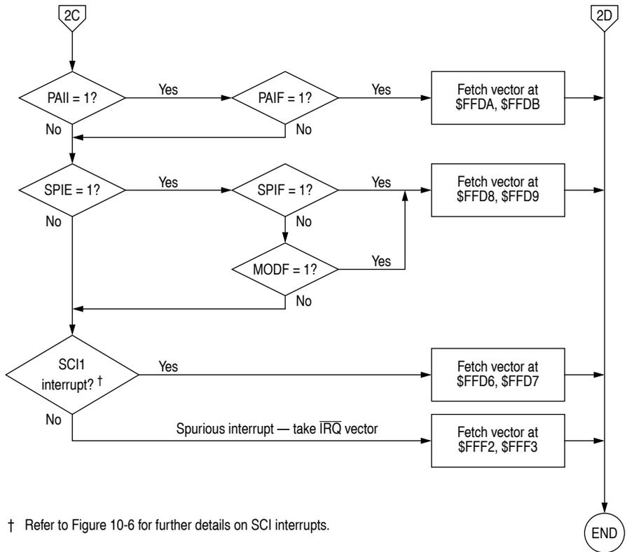
**Figure 10-5** Interrupt priority resolution (3 of 3)
