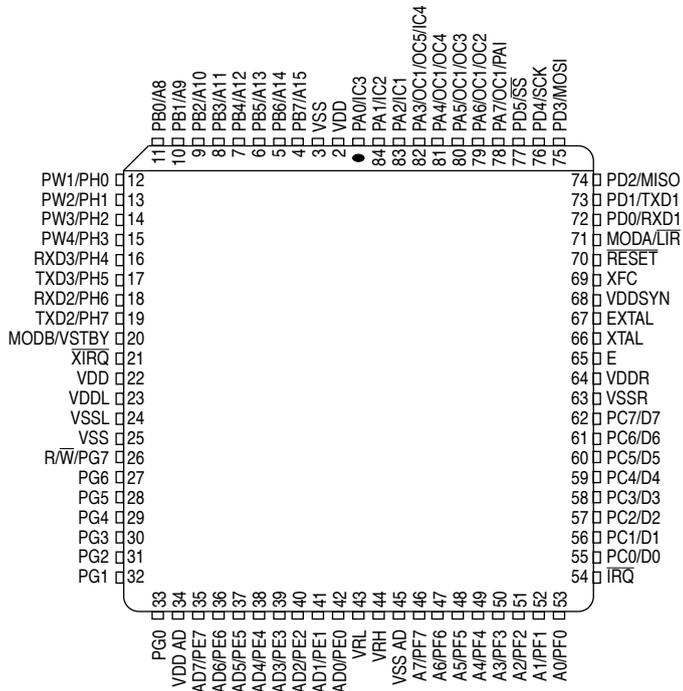
Figure 13-1 84-pin PLCC/CERQUAD pinout
