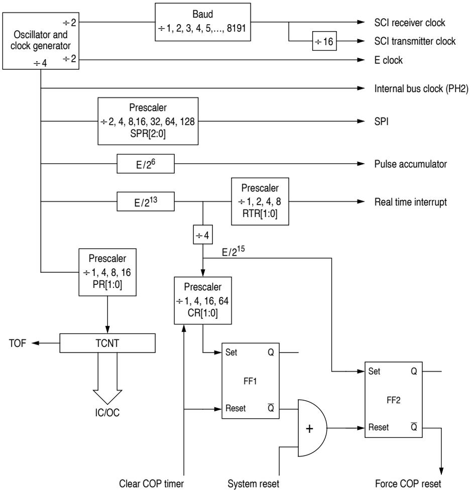
**Figure 8-1** Timer clock divider chains
