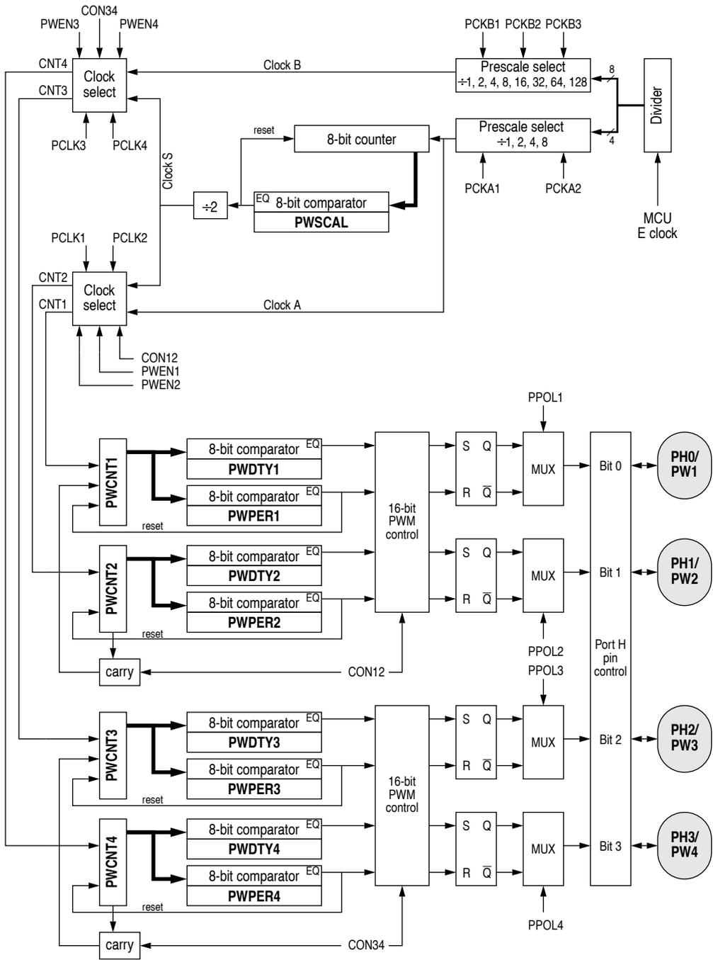
Figure 8-4 PWM timer block diagram
