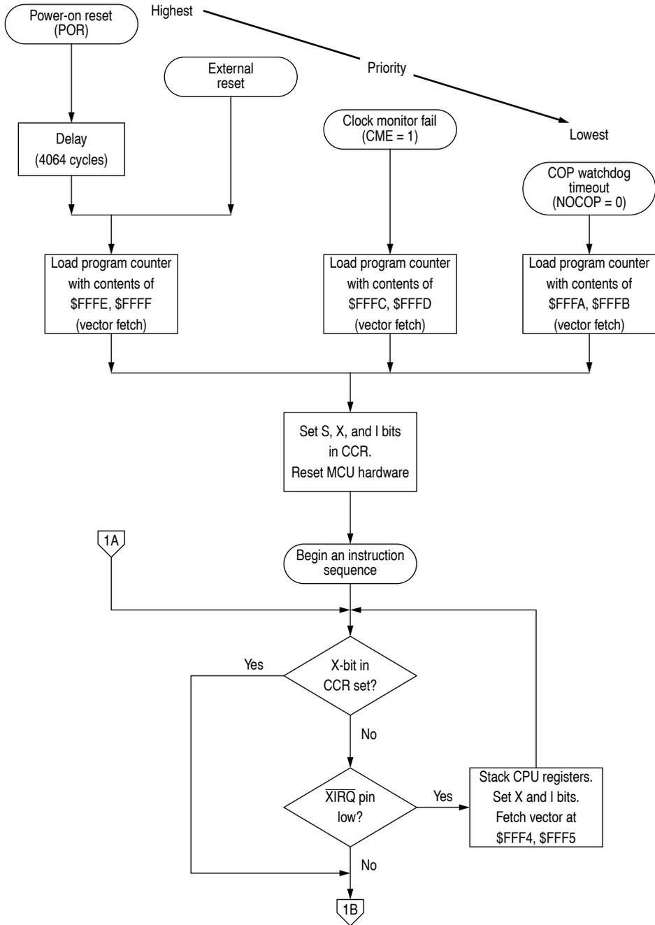
Figure 10-1 Processing flow out of reset (1 of 2)
