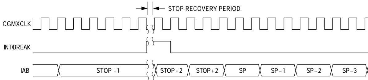
**Figure 16. Stop Mode Recovery from Interrupt or Break**
