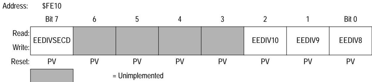
**Figure 5. EEPROM-2 Divider High Non-volatile Register (EEDIVHNVR)**
