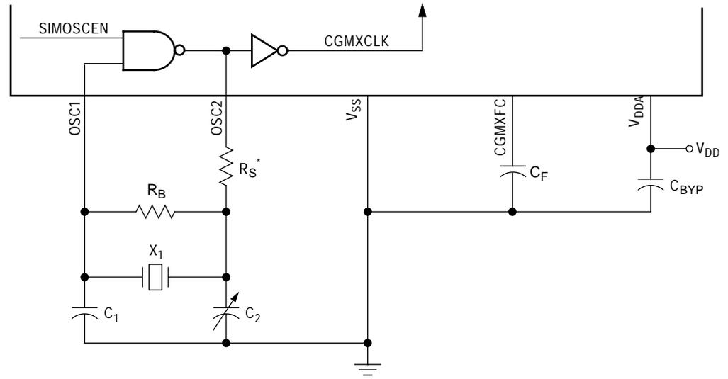
\* $R_S$  can be 0 (shorted) when used with higher-frequency crystals. Refer to manufacturer's data.
