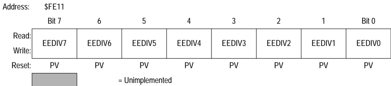
**Figure 6. EEPROM-2 Divider Low Non-volatile Register (EEDIVLNVR)**
