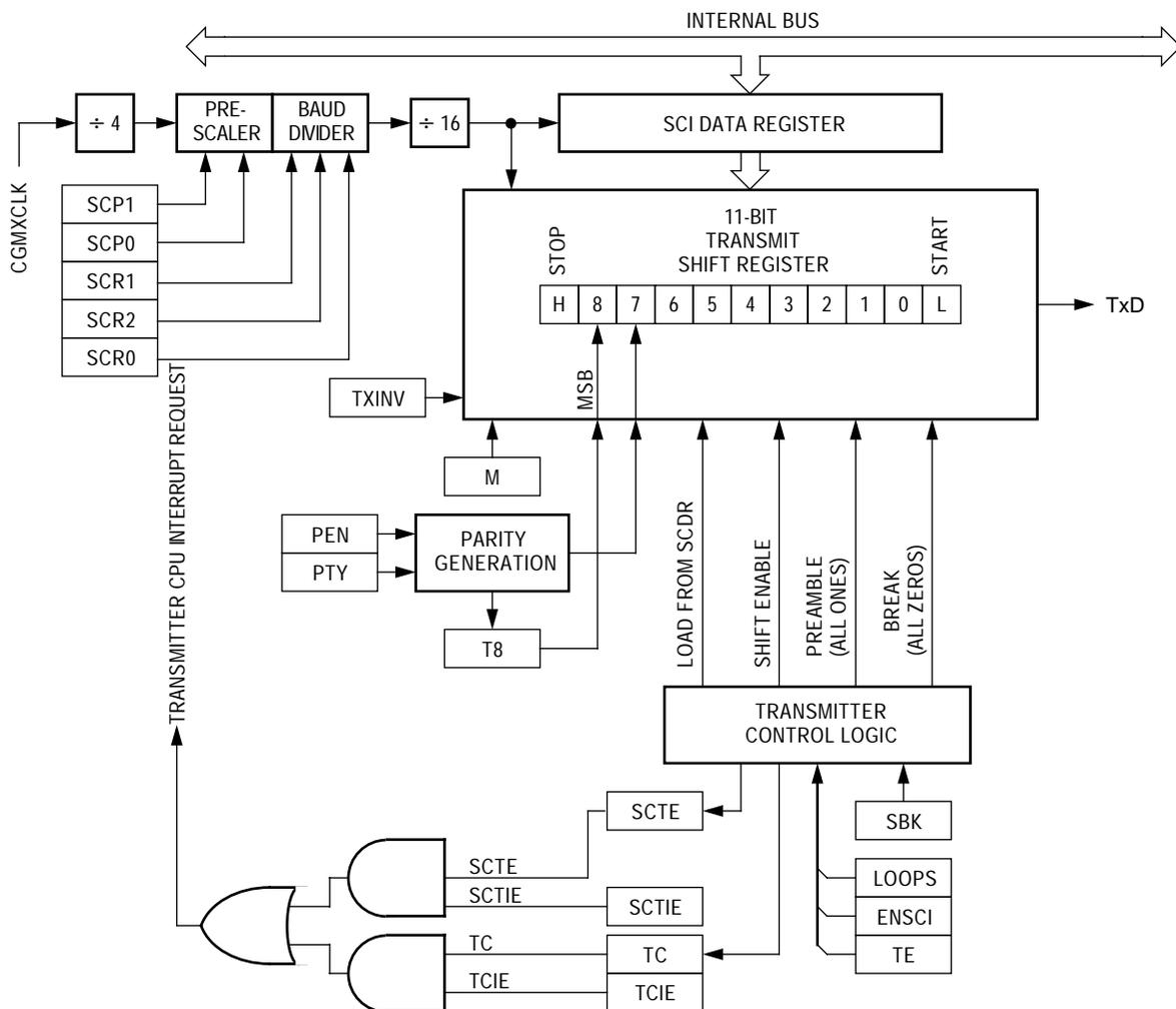
**Figure 4. SCI Transmitter**
