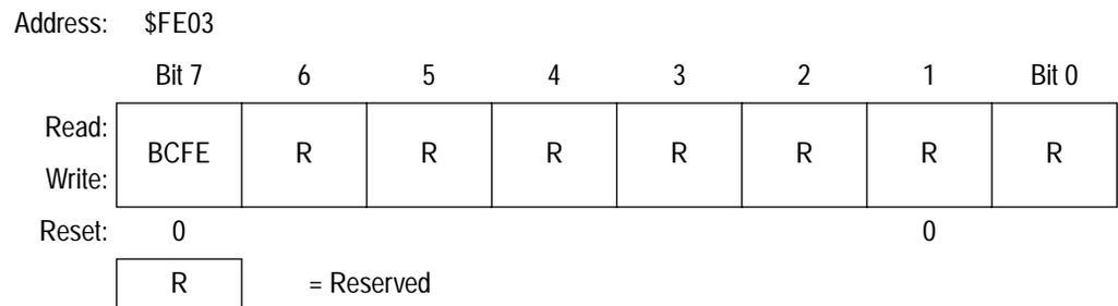
**Figure 19. SIM Break Flag Control Register (SBFCR)**
