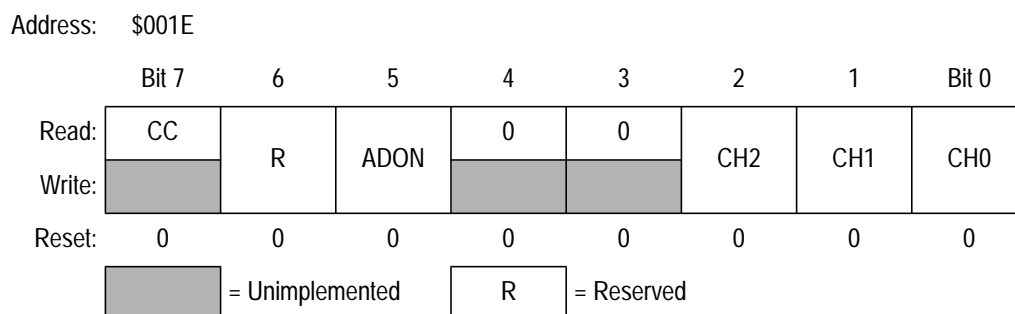
Figure 9-1. A/D Status and Control Register (ADSC)
