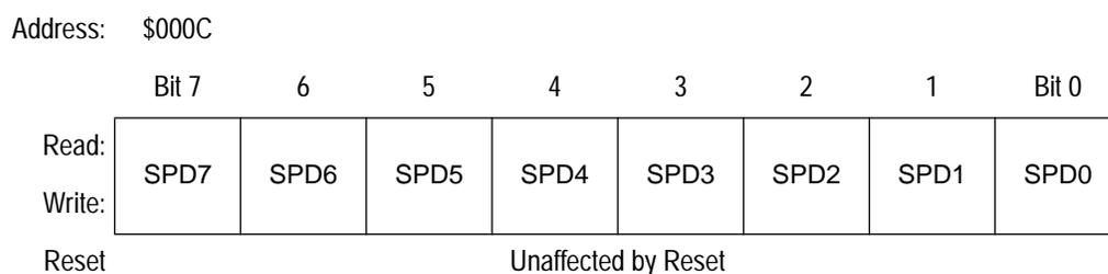
**Figure 10-6. SPI Data Register (SPSR)**
