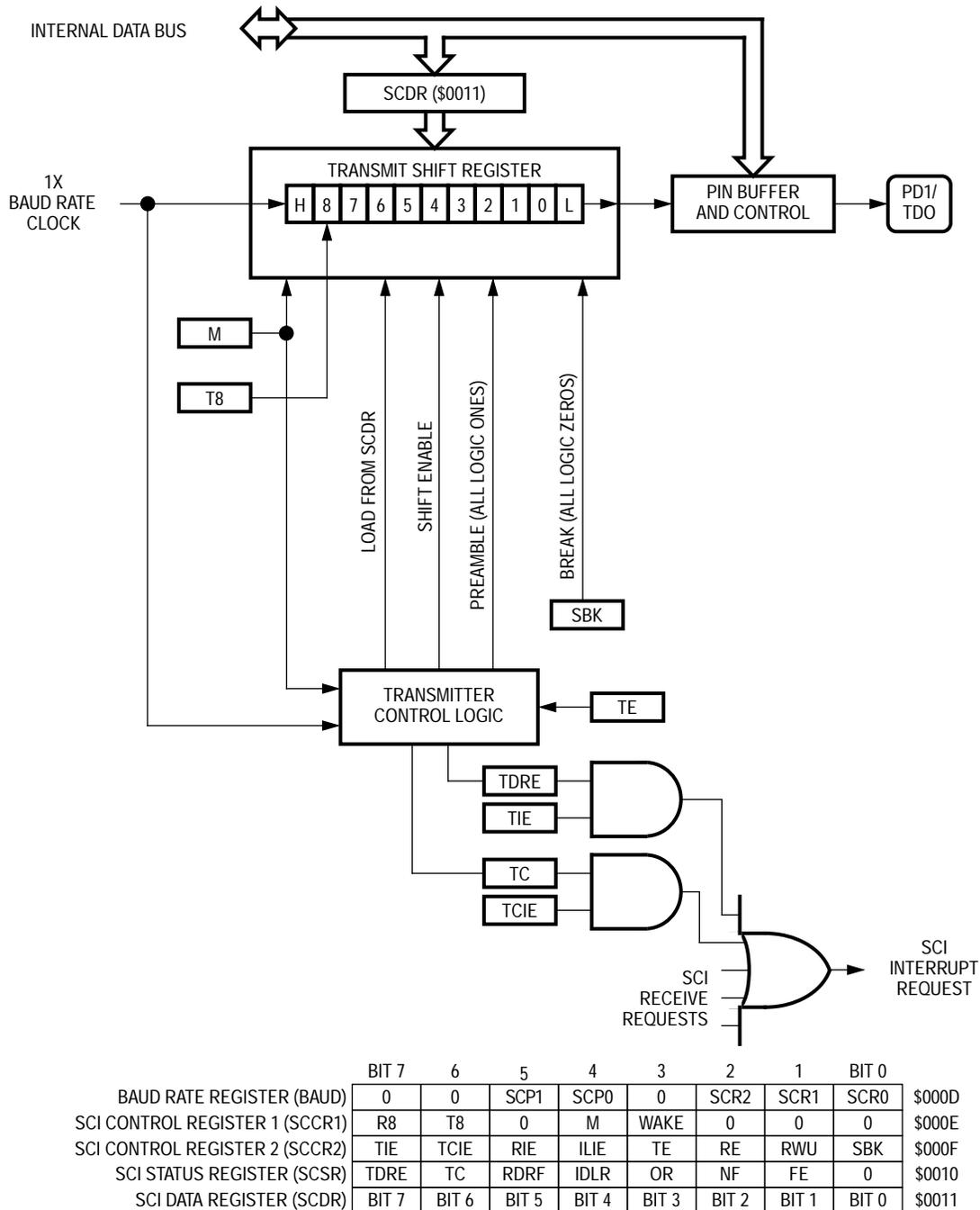
**Figure 9-2. SCI Transmitter**
