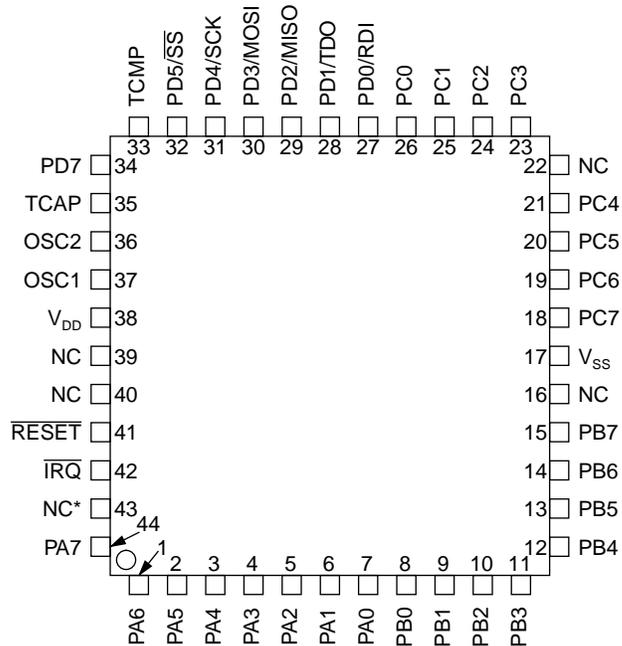
\* If MC68HC705C8A OTPs are to be used in the same application, this pin should be tied to  $V_{DD}$ .
