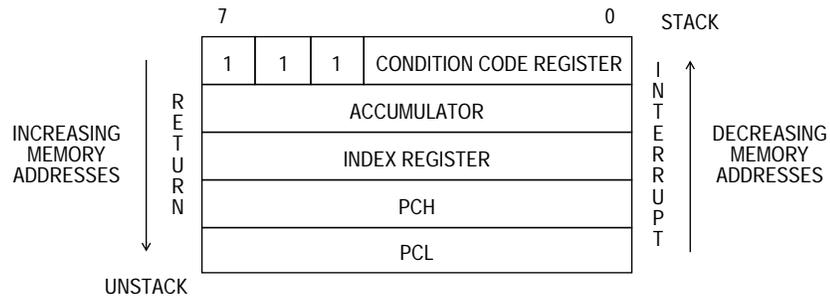
NOTE: Since the stack pointer decrements during pushes, the PCL is stacked first, followed by PCH, etc. Pulling from the stack is in the reverse order.
