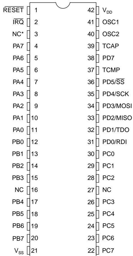
\* If MC68HC705C8A OTPs are to be used in the same application, this pin should be tied to V<sub>DD</sub>.
