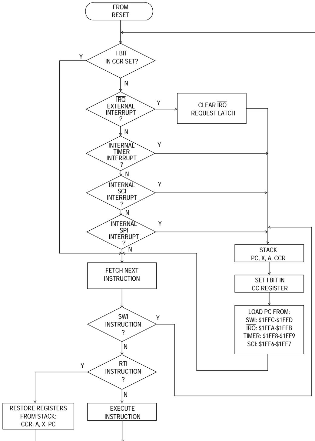
**Figure 4-1. Interrupt Flowchart**
