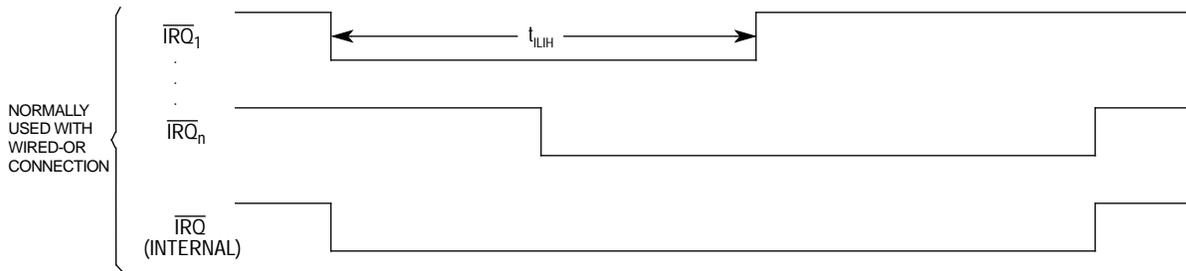
**b. Level-Sensitive Trigger Condition.** If after servicing an interrupt the  $\overline{IRQ}$  remains low, the next interrupt is recognized.
