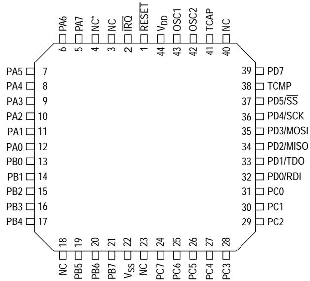
\* If MC68HC705C8A OTPs are to be used in the same application, this pin should be tied to  $V_{DD}$ .
