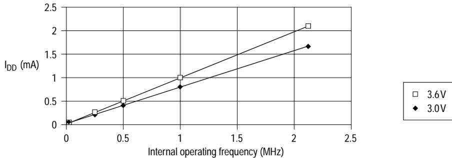
Figure 11-7 Run I<sub>DD</sub> vs internal operating frequency (3V, 3.6V)
