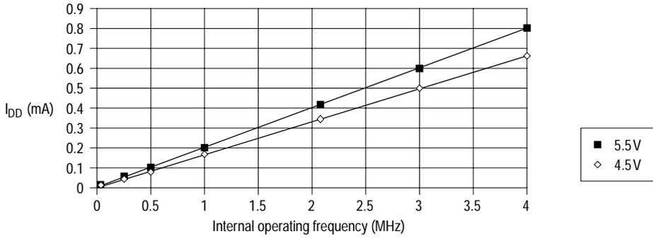
**Figure 11-4** Wait I<sub>DD</sub> (SM = 1) vs internal operating frequency (4.5V, 5.5V)
