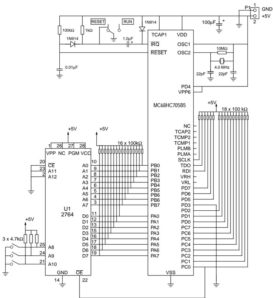
Figure C-8 RAM parallel bootstrap schematic diagram
