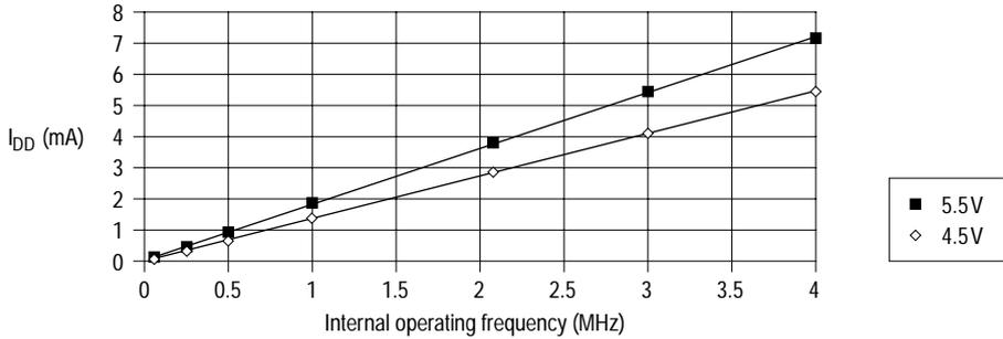
**Figure 11-1** Run I<sub>DD</sub> vs internal operating frequency (4.5V, 5.5V)
