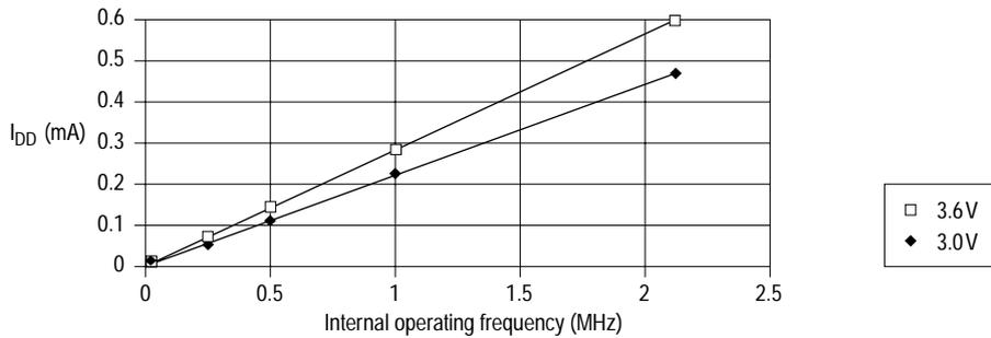
Figure 11-8 Run I<sub>DD</sub> (SM = 1) vs internal operating frequency (3V, 3.6V)
