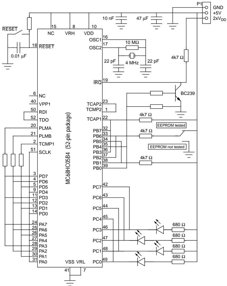
*Note:* For the MC68HC05B4, switches on PB5 and PB6 have no effect
