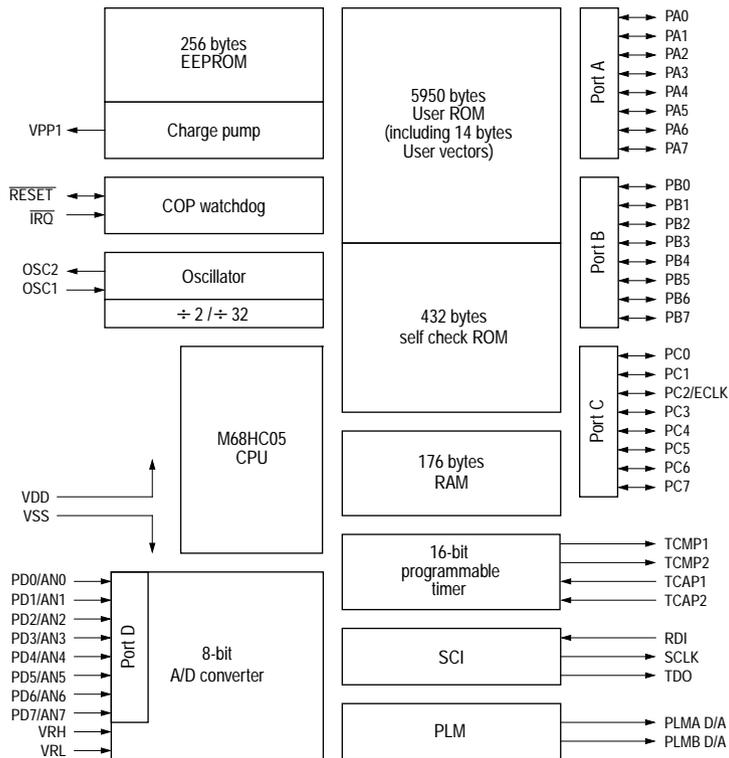
Figure 1-1 MC68HC05B6 block diagram
