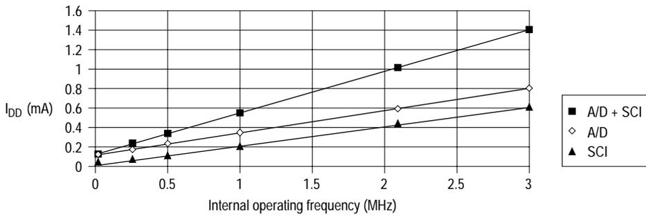
**Figure 11-5** Increase in I<sub>DD</sub> vs frequency for A/D, SCI systems active, V<sub>DD</sub> = 5.5V
