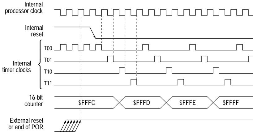
*Note:* The counter and timer control registers are the only ones affected by power-on or external reset.
