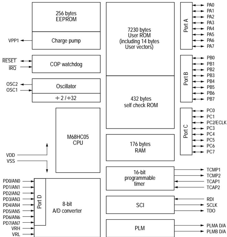
**Figure B-1** MC68HC05B8 block diagram
