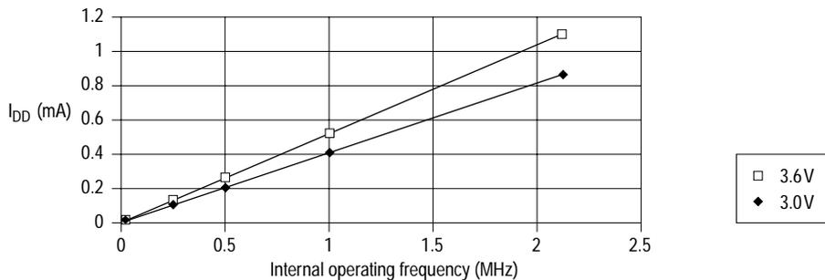
Figure 11-9 Wait I<sub>DD</sub> vs internal operating frequency (3V, 3.6V)
