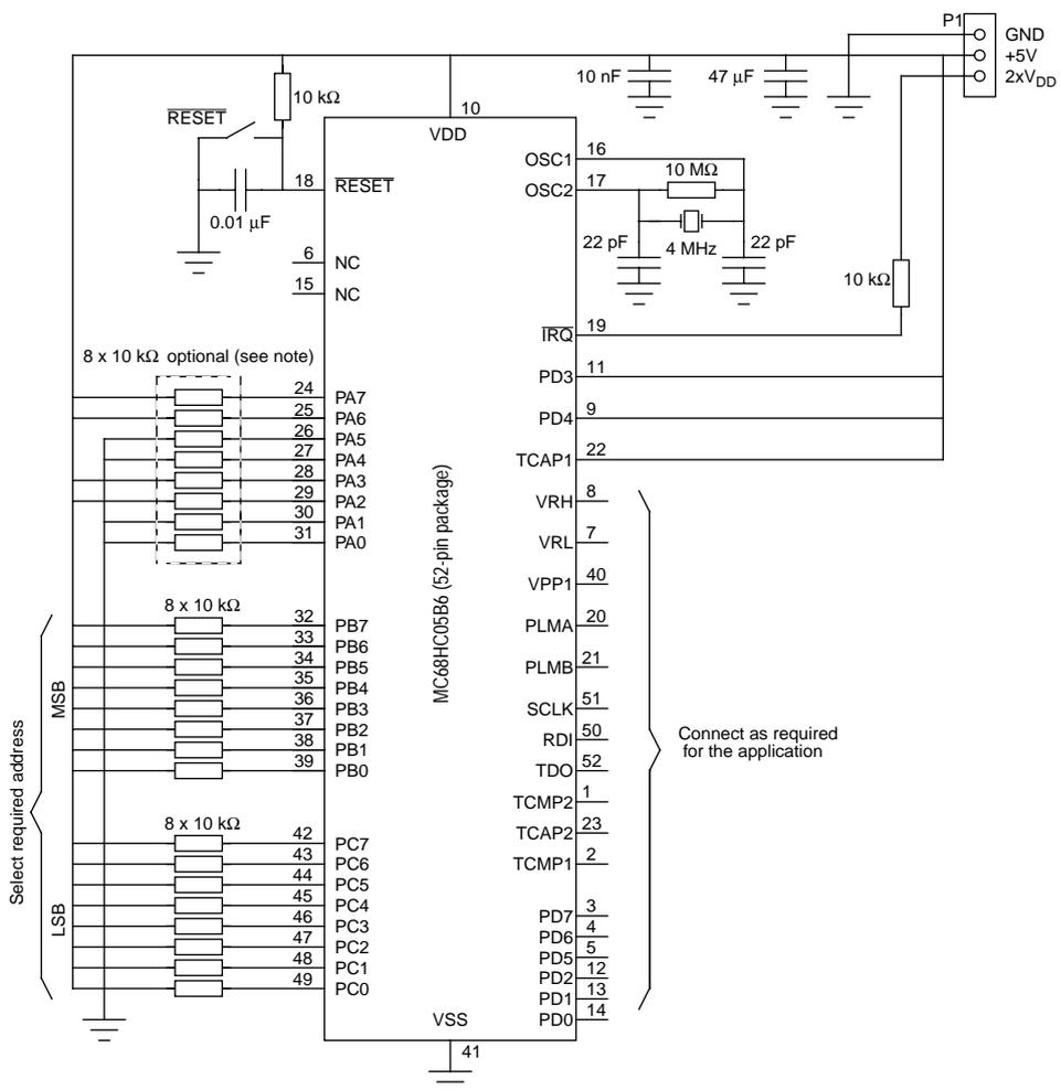
*Note:* These eight resistors are optional: direct connection is possible if pins PA0-PA7, PB0-PB7 and PC0-PC7 are kept in input mode during application.
