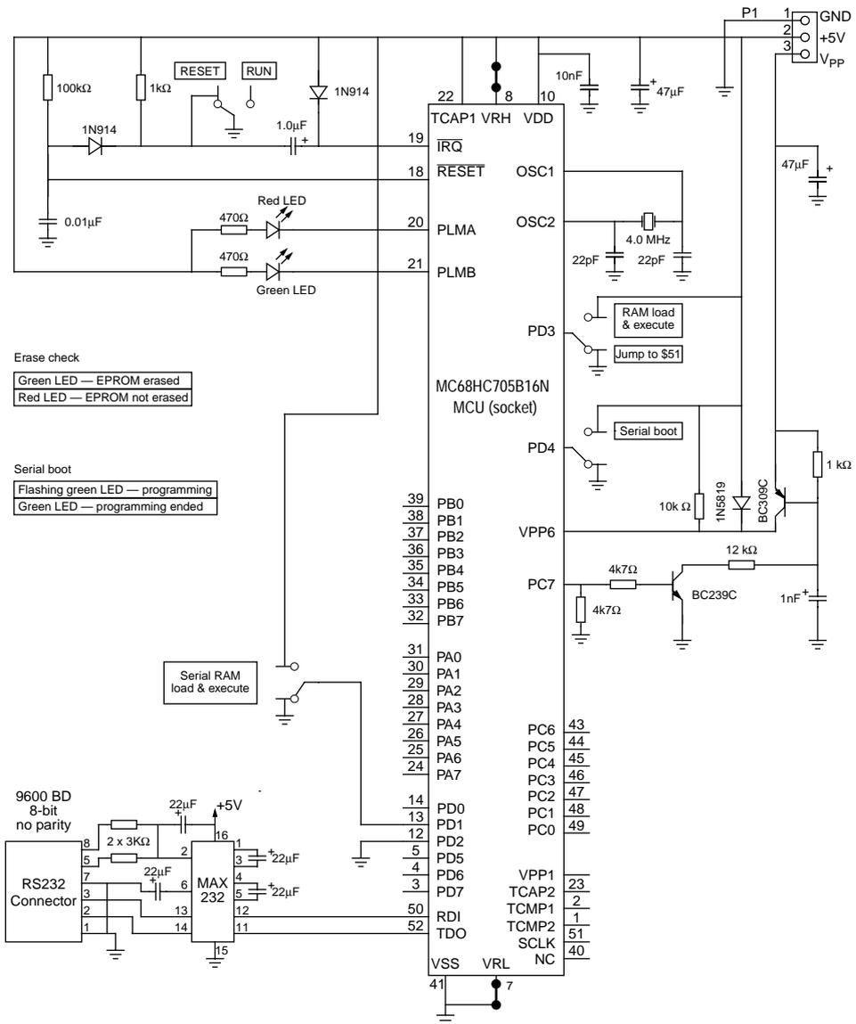
**Note:** A minimum  $V_{DD}$  voltage must be applied to the VPP6 pin at all times, including power-on, as a lower voltage could damage the device. Unless otherwise stated, EPROM programming is guaranteed at ambient (25°C) temperature only
