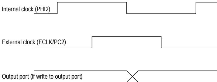
Figure 4-2 ECLK timing diagram
