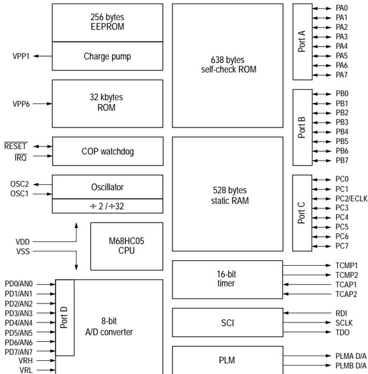
**Figure G-1** MC68HC05B32 block diagram
