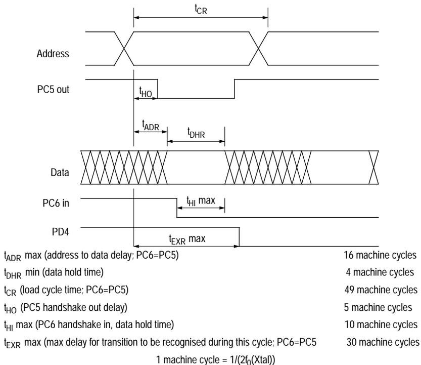
Figure E-9 Parallel RAM loader timing diagram
