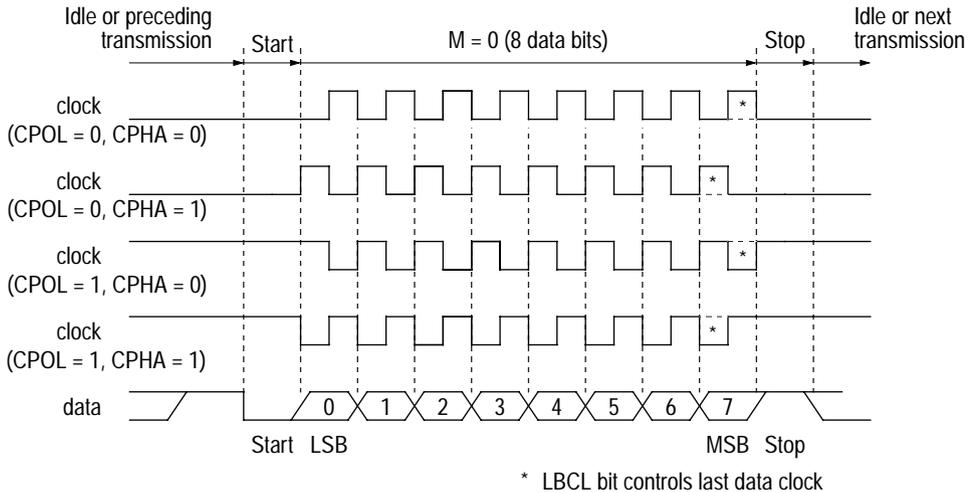
**Figure 6-9** SCI data clock timing diagram (M=0)
