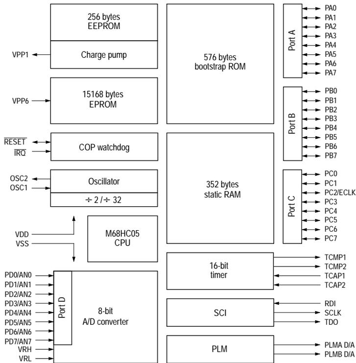
**Figure E-1** MC68HC705B16 block diagram
