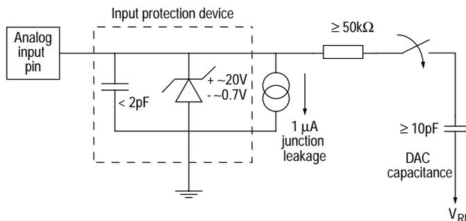
*Note:* The analog switch is closed during the 12 cycle sample time only.
