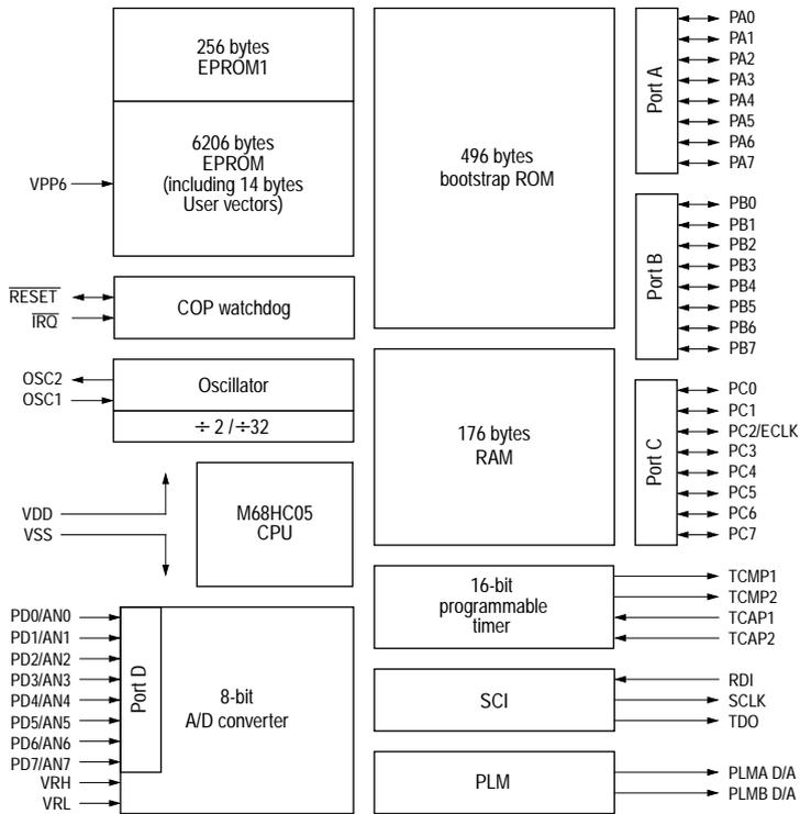
**Figure C-1** MC68HC705B5 block diagram
