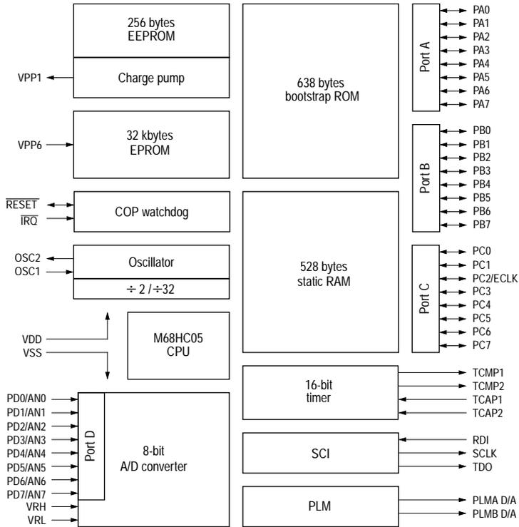
**Figure H-1** MC68HC705B32 block diagram
