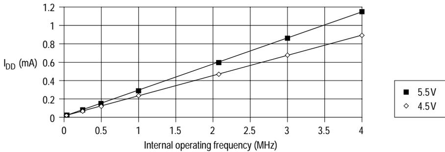
**Figure 11-2** Run I<sub>DD</sub> (SM = 1) vs internal operating frequency (4.5V, 5.5V)
