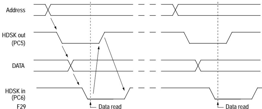
Figure C-5 Timing diagram with handshake
