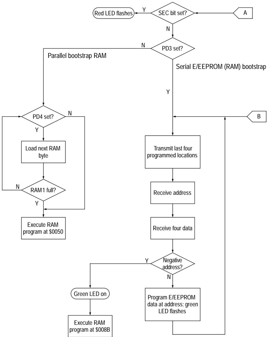
**Figure E-4** Modes of operation flow chart (2 of 2)
