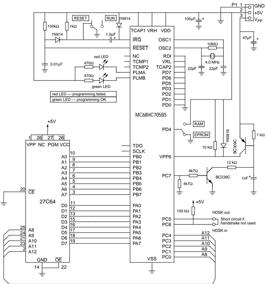
**Note:** This circuit is recommended for programming only at 25°C and not for use in the end application, or at temperatures other than 25°C. If used in the end application, VPP6 should be tied to VDD to avoid damaging the device.
