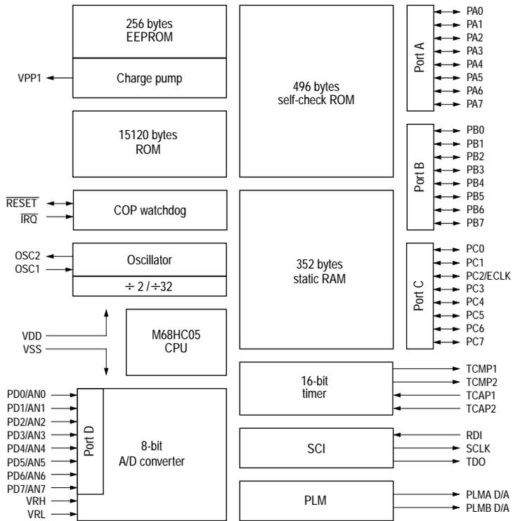
Figure D-1 MC68HC05B16 block diagram
