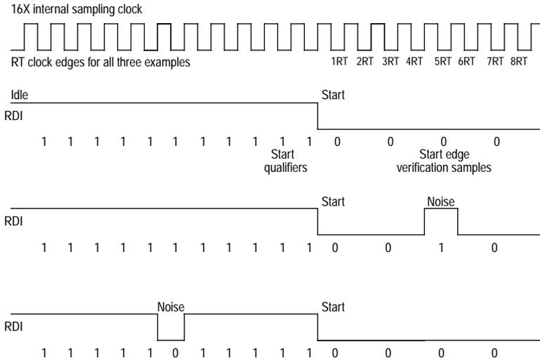
**Figure 6-4** SCI examples of start bit sampling technique
