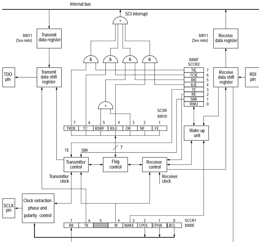
*Note:* The serial communications data register (SCI SCDR) is controlled by the internal R/W signal. It is the transmit data register when written to and the receive data register when read.
