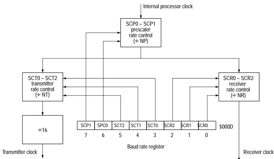
*Note:* There is a fixed rate divide-by-16 before the transmitter to compensate for the inherent divide-by-16 of the receiver (sampling). This means that by loading the same value for both the transmitter and receiver baud rate selector, the same baud rates can be obtained.
