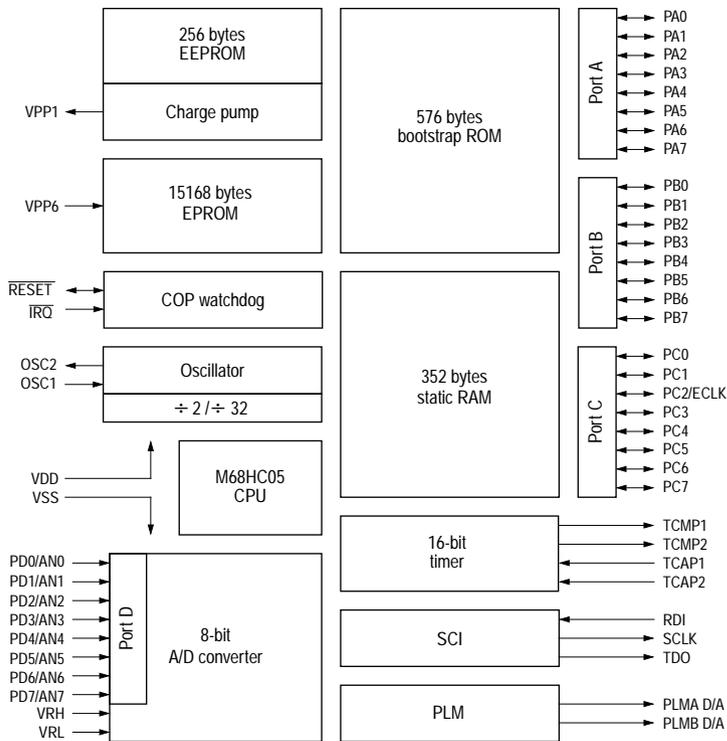
Figure F-1 MC68HC705B16N block diagram
