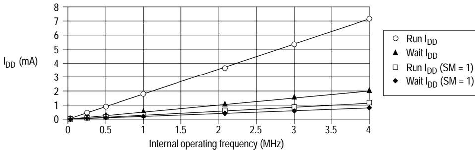
**Figure 11-6** I<sub>DD</sub> vs mode vs internal operating frequency, V<sub>DD</sub> = 5.5V
