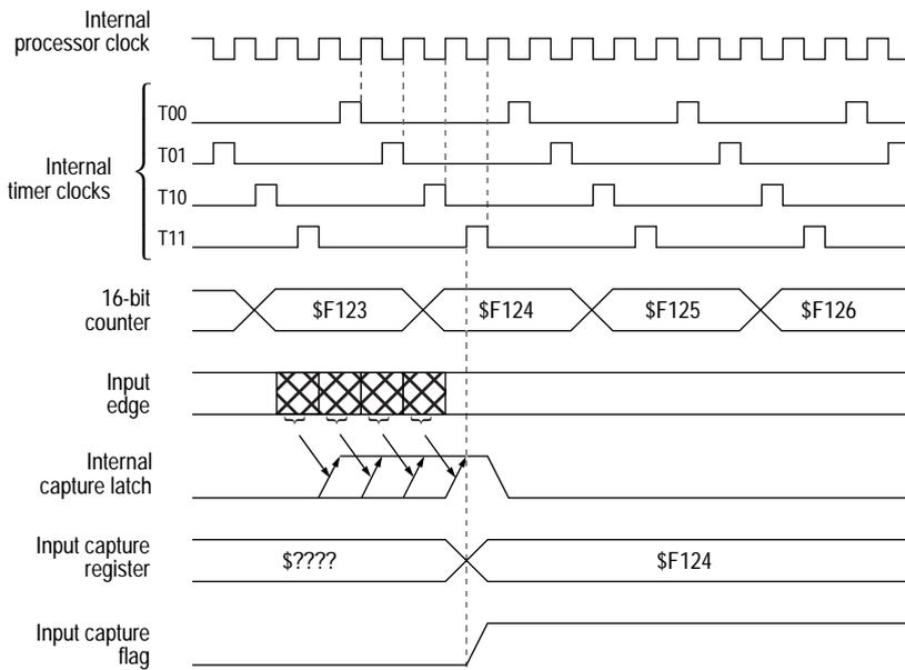
*Note:* If the input edge occurs in the shaded area from one timer state T10 to the next timer state T10, then the input capture flag will be set during the next T11 state.
