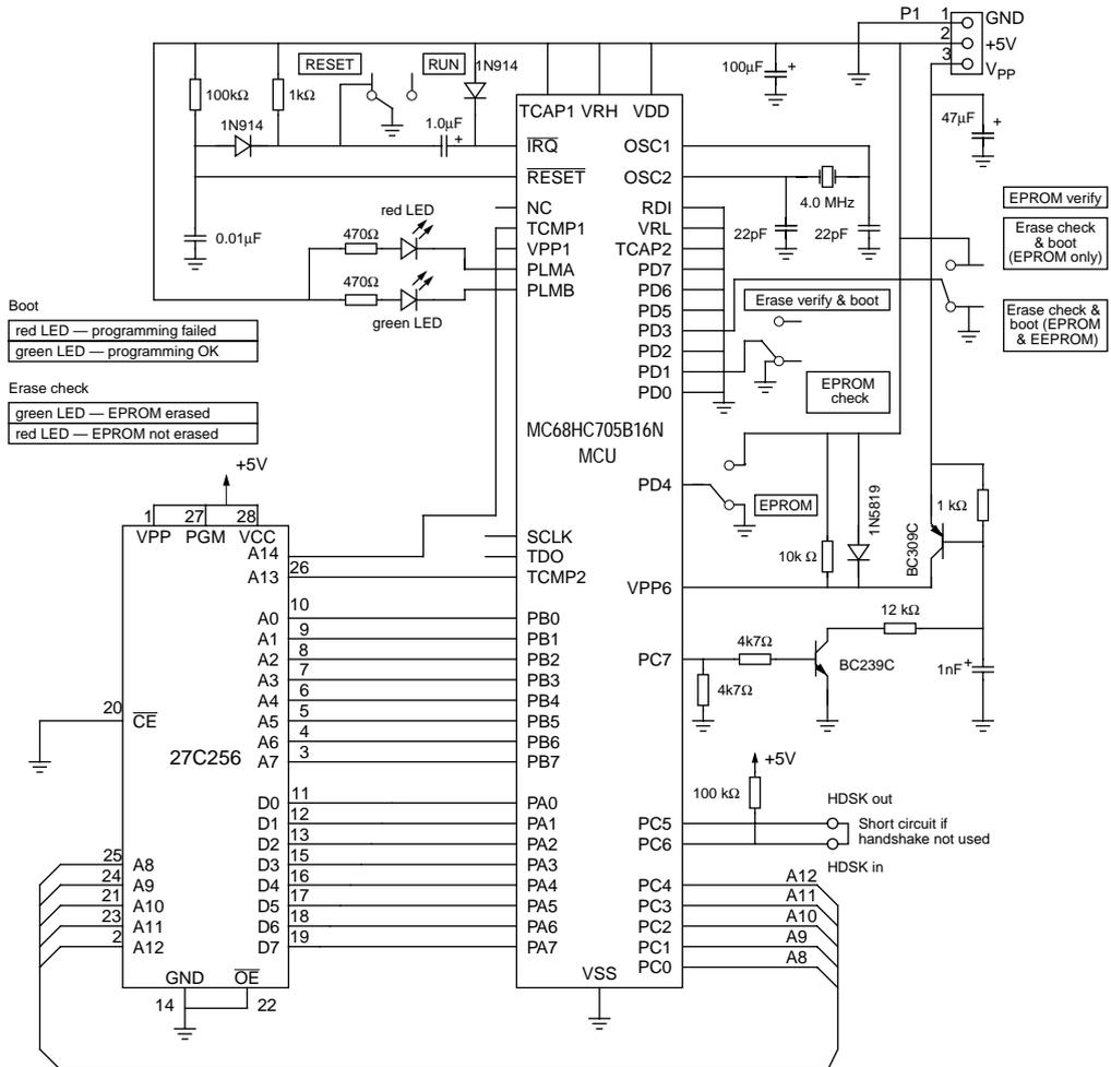
**Note:** This circuit is recommended for programming only at 25°C and not for use in the end application, or at temperatures other than 25°C. If used in the end application, VPP6 should be tied to VDD to avoid damaging the device.
