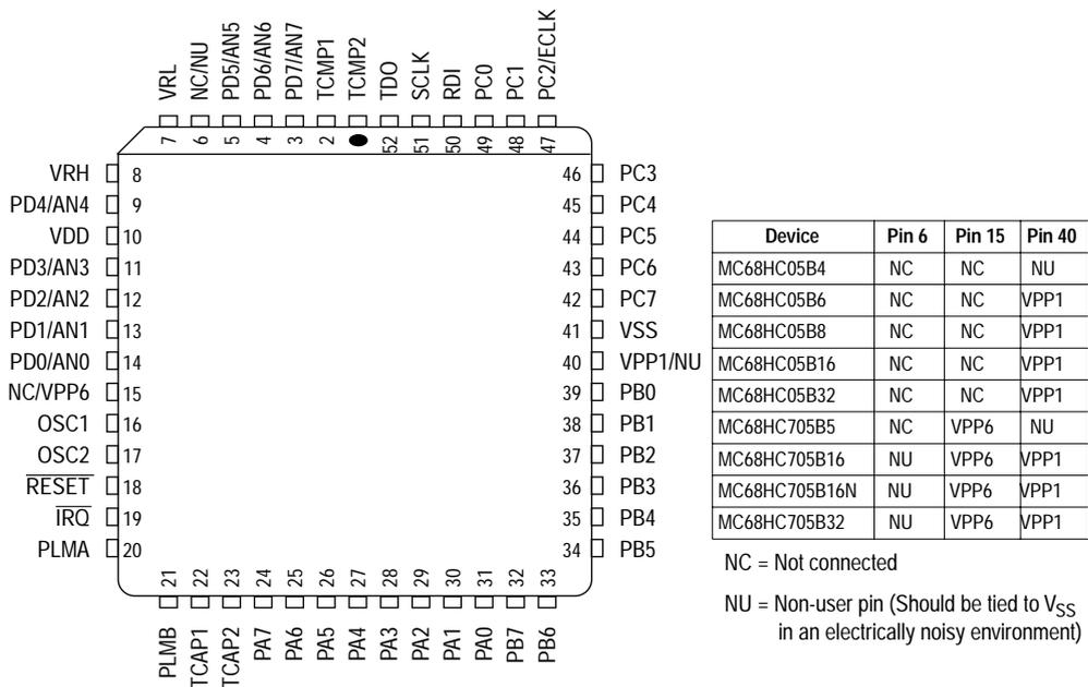
Figure 12-1 52-pin PLCC pinout for the MC68HC05B6
